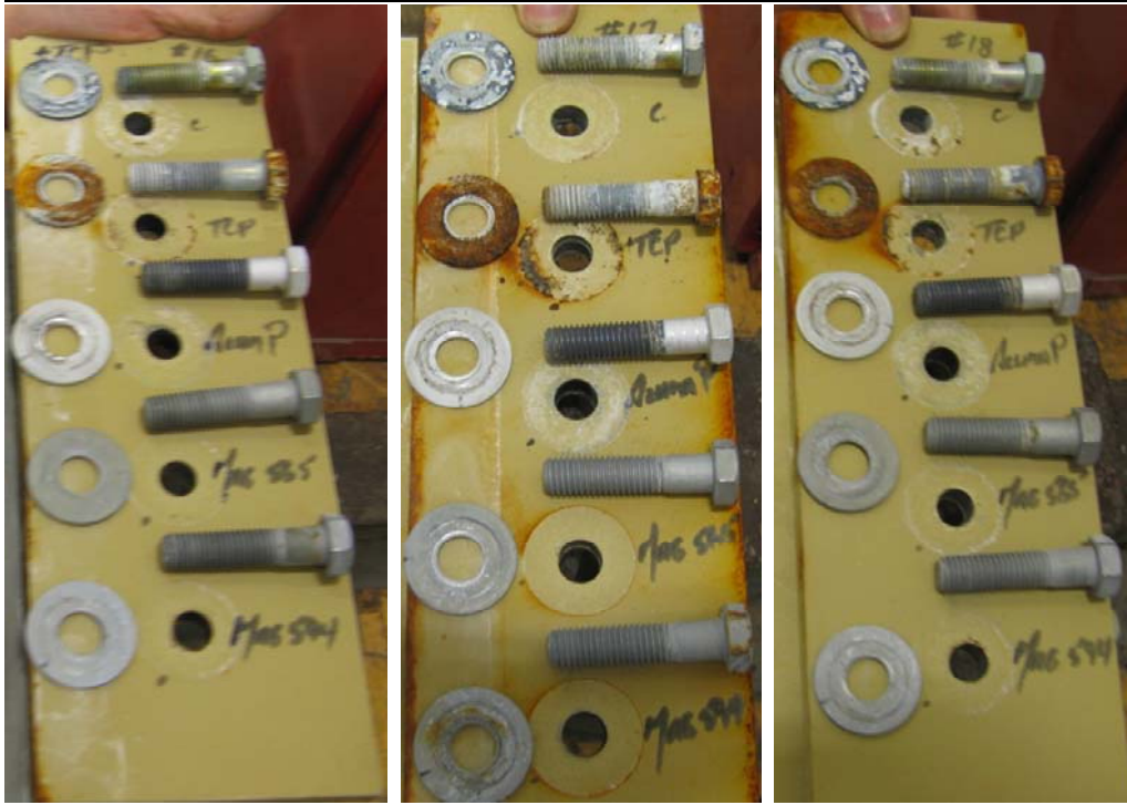
Figure A-7. Panels 16, 17, and 18 disassembled after 120 cycles GM9540P.
