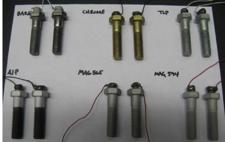
Figure 2. Prepared bolts prior to immersion in thermostatic bath.
