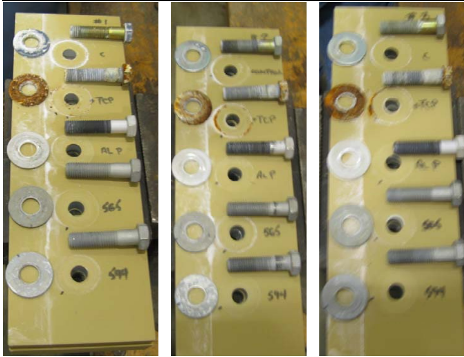
Figure A-1. Plates 1–3 disassembled after 120 cycles GM9540P.
