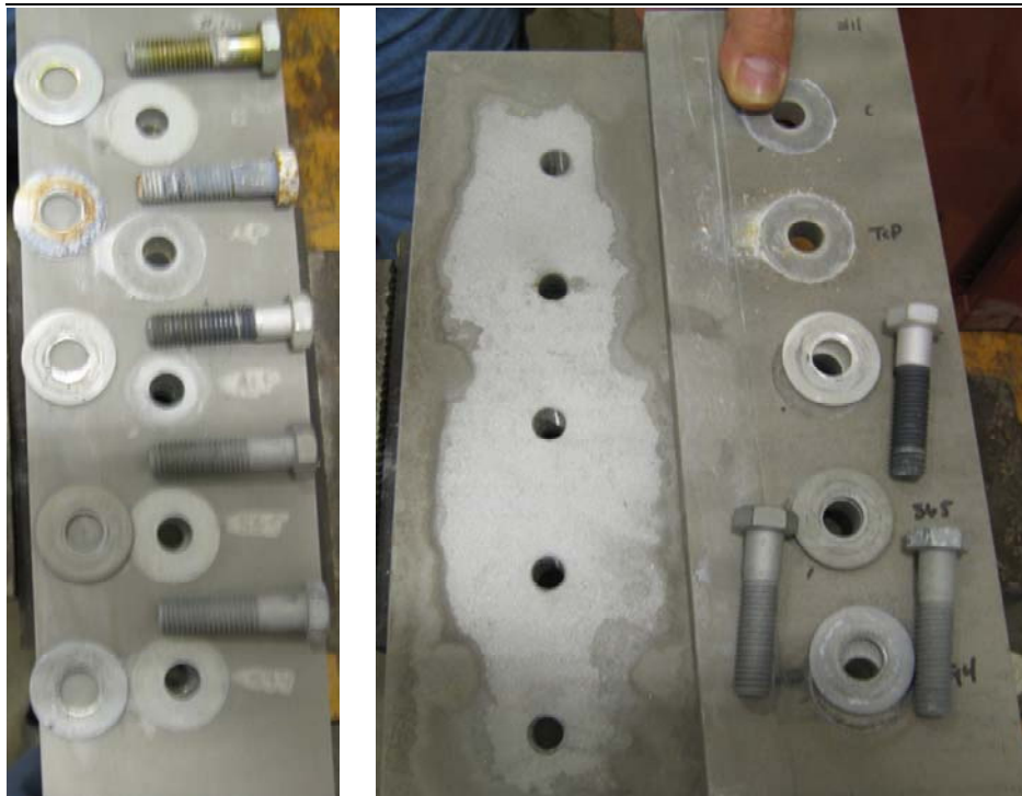
Figure A-4. Panels 10 and 11 disassembled after 120 cycles GM9540P (including interior shot to show moisture penetration on panel 11).
