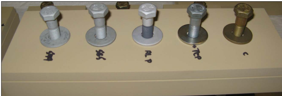
Figure 5. Photograph of plate assembly prior to final assembly (from left to right: Magniplate 594, Magniplate 565, Alumiplate, TCP, Hexavalent chrome).
