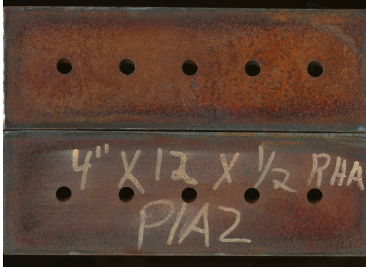
Figure 3. RHA steel prior to surface finishing.
