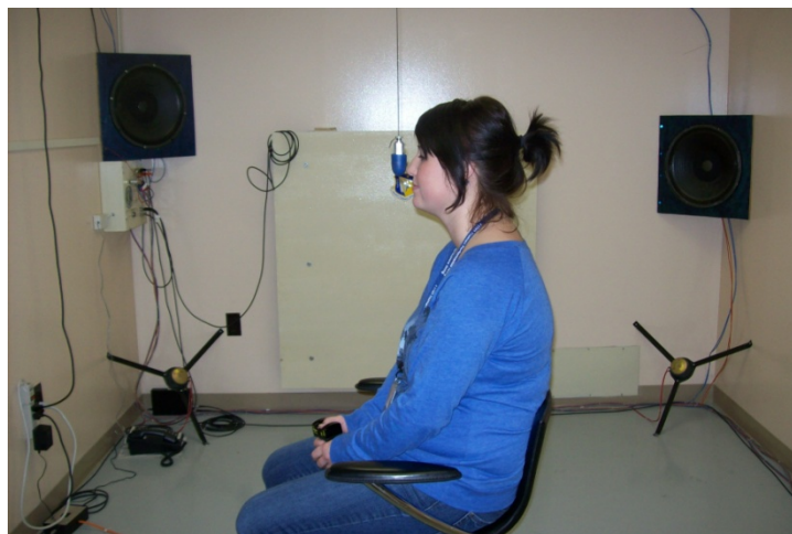
Figure 2. Female subject in REAT facility, open ear condition
