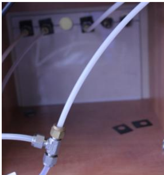
Figure 21. This picture shows the Tee used to combine two different gases to be used for making the aerosol.
