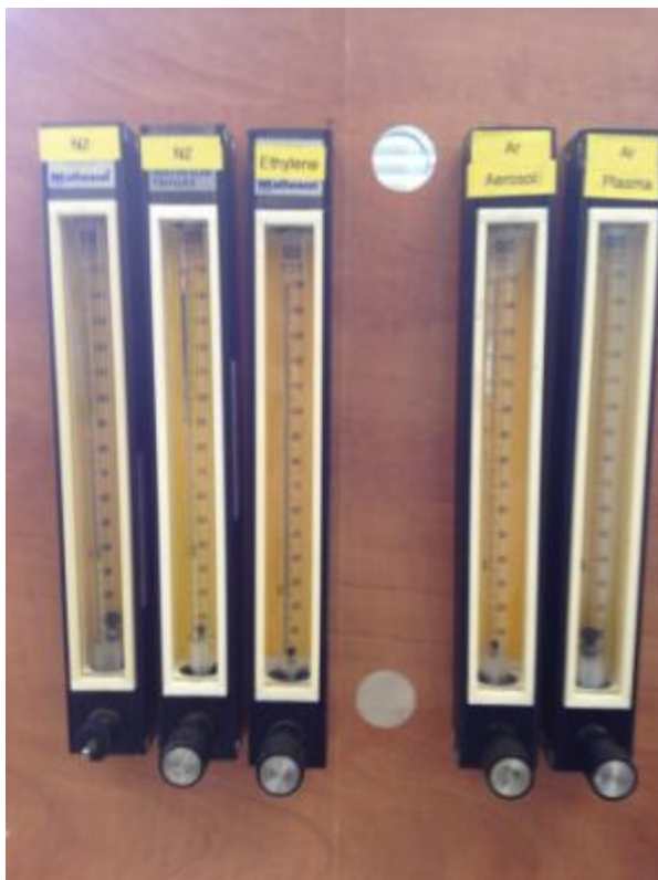
Figure 18. This is a picture of the flow meters used for the system.
