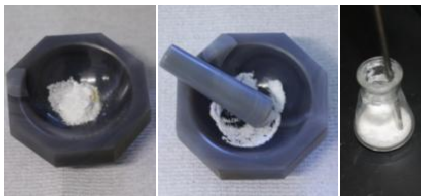
Figure 16. This figure shows the process used to prepare a precursor from left to right. It involves measuring the precursors, crushing them into a fine powder, and then drying them using nitrogen gas.
