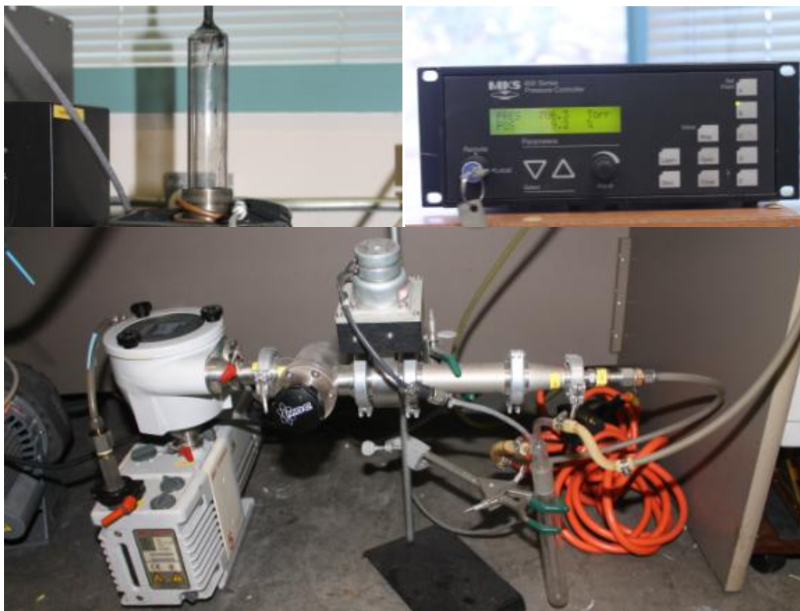
Figure 20. Top left shows the chimney when it is attached, the top right shows the MKS controller used to regulate system pressure, and the bottom shows the pump and control valve used to exhaust the gases.
