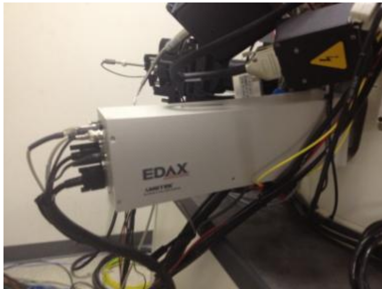
Figure 27. This is a picture of the EDAX Pegasus system.
