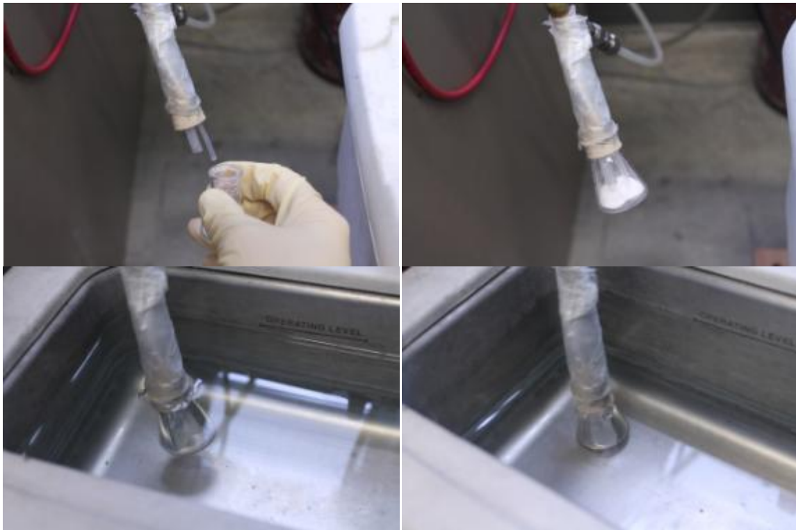
Figure 17. This is a depiction of loading the sample into the system and adjusting the water level of the sonic bath.
