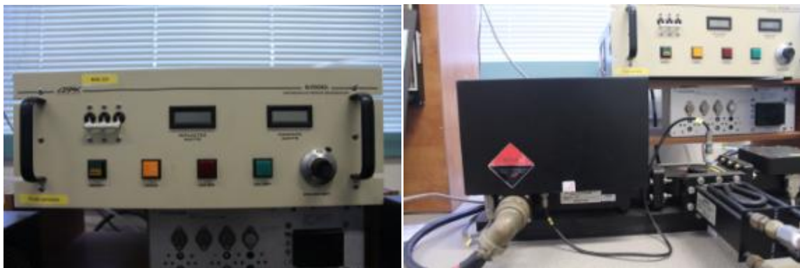
Figure 10. On the left is the power supply and on the right is the magnetron.
