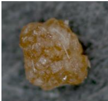
Figure 9. Prill after being heated at 175 °C for the GC-MS analysis.
