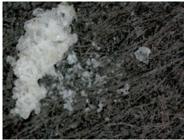
Figure 2. Image of "smeared" Comp A-3 prill taken with an optical microscope.
