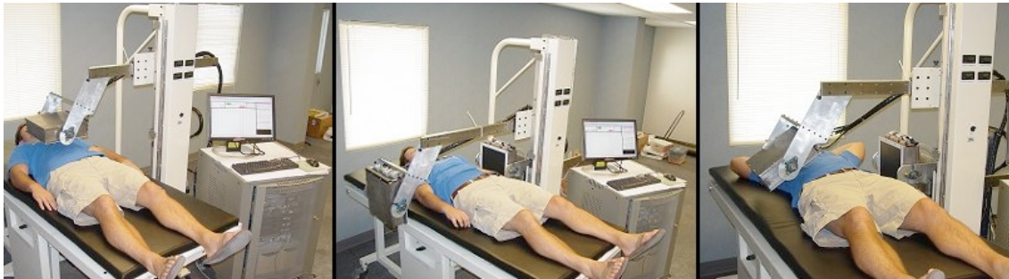
Fig. 7: Photograph of system gantry with actual detectors mounted. Detectors are positioned in anterior/posterior (left), lateral (middle), and both anterior (right) orientations
