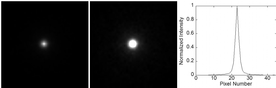
Fig. 15. GATE simulation of a point source and the pinhole hole collimator without windowing (left), windowed to 25% of the maximum pixel intensity (middle), and a horizontal profile (right). Notice that there are penetration photons but there is no star pattern.
