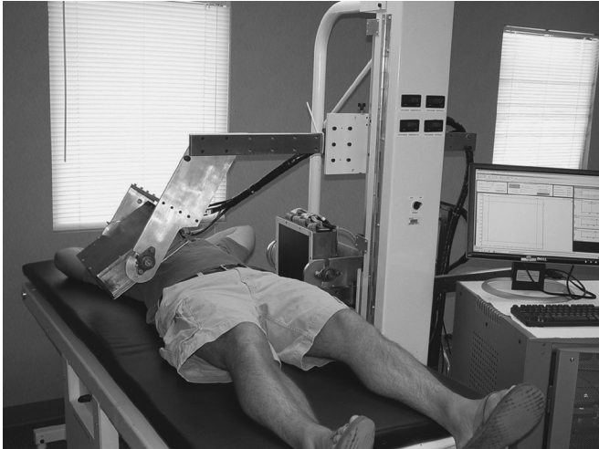
Fig. 1. Photograph of bedside cardiac imaging system. Detectors are shown in left lateral and right anterior oblique orientations. Associated electronics rack and computers shown at right.
