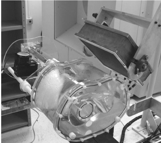
Fig. 2. The dynamic cardiac phantom and the bedside imaging system with the detector head in a left oblique position (45 degrees).
