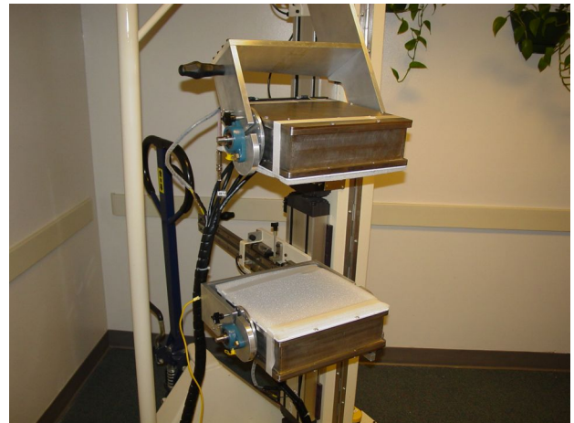
Fig. 1. Photograph of 25 cm x 25 cm detector heads attached to mobile gantry installed at the University of Florida.
