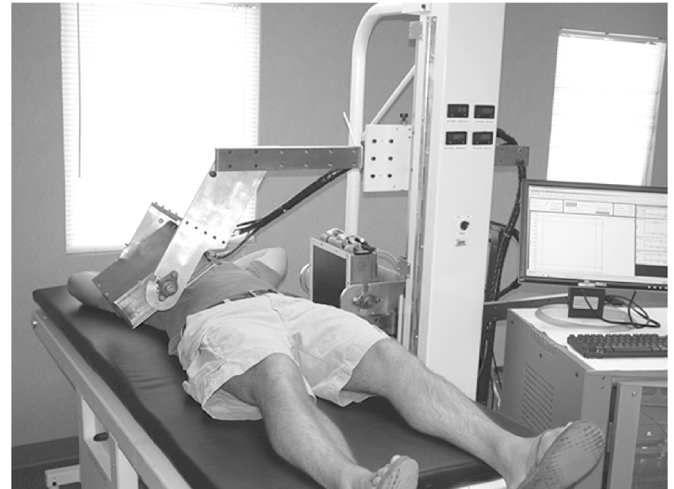
Fig. 1. Mobile gantry with detectors in an oblique and lateral orientation for SPECT imaging along with the associated mobile electronics rack seen to the right.
