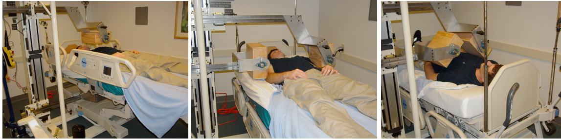
Fig. 2: Photographs of system gantry with mock detectors positioned in anterior/posterior opposing (left), lateral opposing (center), and anterior “L” orientations.
