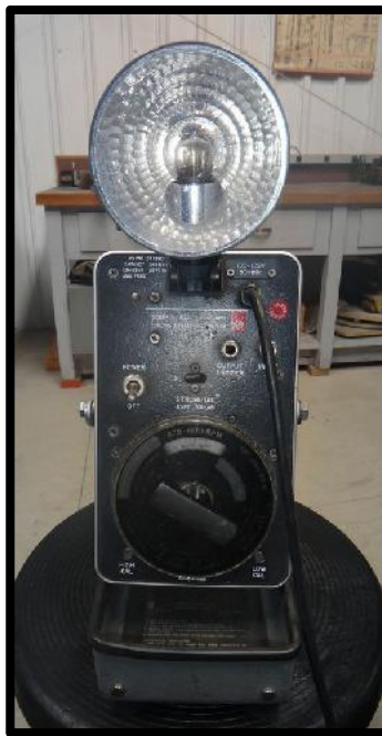
Figure 23. Strobe tachometer used to measure speed.
