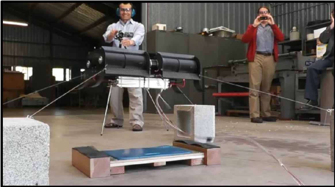
Figure 42. Successful lift-off of four rotor chassis.
