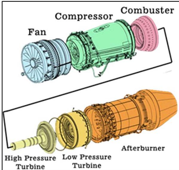
Figure 4. Six Sections of the F414-GE-400 Engine
