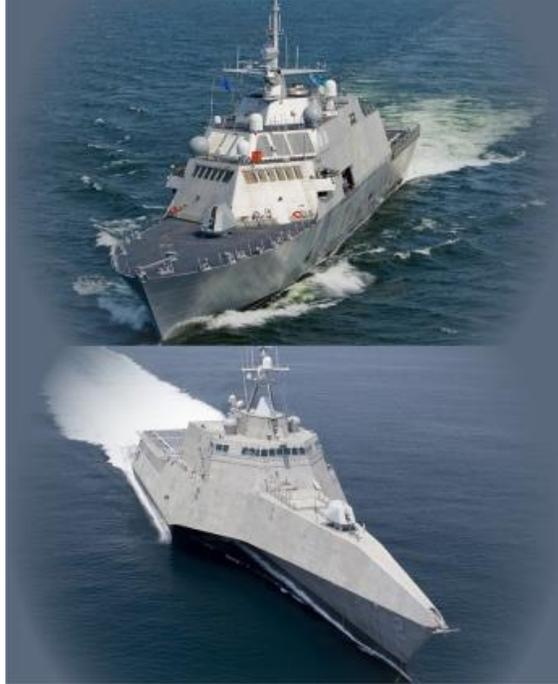
Figure 2. LCS-1 (above) - Lockheed Martin's design of aluminum superstructure and steel hull; LCS-2 (below) - General Dynamics' design of an all-aluminum alloy hull. From *LCS: The USA's Littoral Combat Ships* (From [10]).
