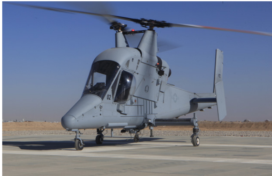
Figure 44. Lockheed Martin K-max UAS.
