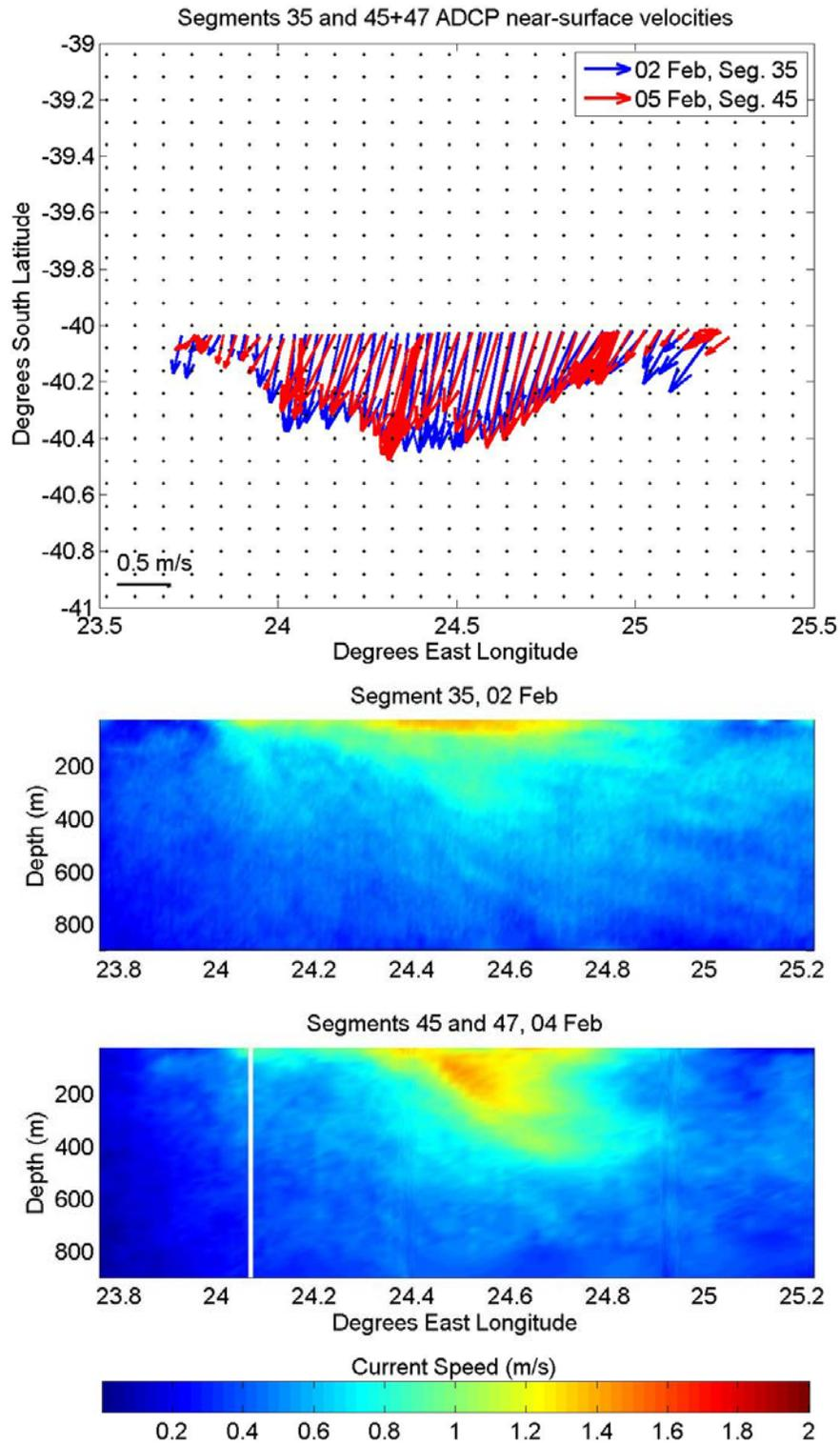
Figure 14. Change in velocities observed near  $40.0^{\circ}\text{S}$ ,  $24.5^{\circ}\text{E}$  from 2 to 4 February. Upper subfigure shows near-surface ADCP velocity vectors, lower subfigures show depth-longitude ADCP speed cross sections.
