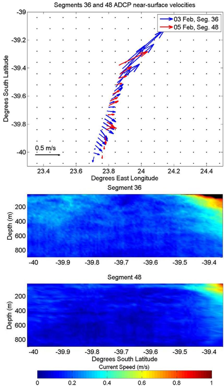
Figure 17. Change in velocities observed near  $39.5^{\circ}\text{S}$ ,  $23.8^{\circ}\text{E}$  from 3 to 5 February. Upper subfigure shows near-surface ADCP velocity vectors, lower subfigures show depth-longitude ADCP speed cross sections. Velocities greater than 1 m/s are shown in black.
