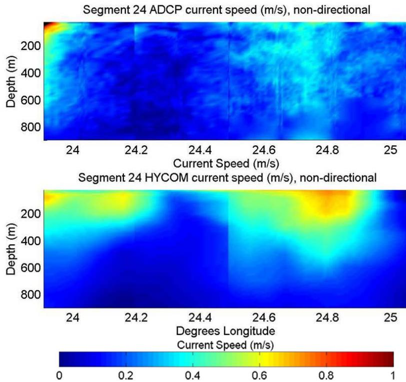
Figure 8. Segment 24 HYCOM and ADCP velocities. Near-surface velocities shown on top, ADCP velocity cross section in middle, and HYCOM velocity cross section at bottom. Velocities greater than 1 m/s are shown in black.
