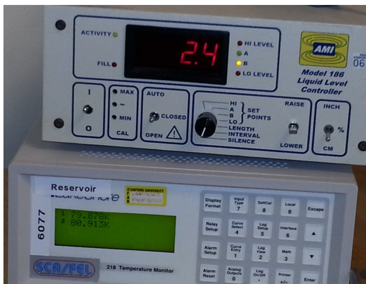
Figure 31. Temperature monitor at 80 K and Liquid level controller.
