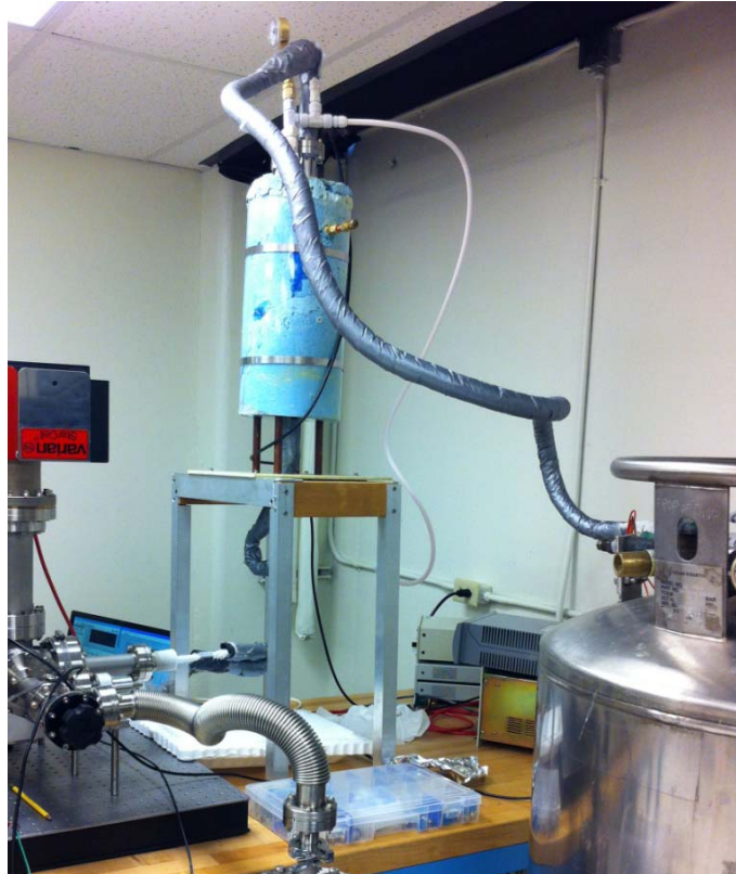
Figure 9. Cathode cooling system connected to LN tank.
