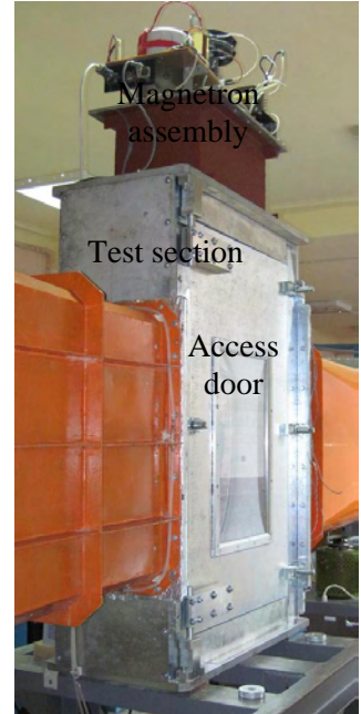
Figure 2.4. Wind-tunnel test section with the MW radiation system on its top
