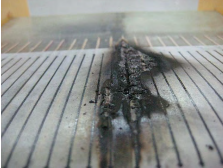
Fig. 3.3. The burn-out of the surface of model #11_2
