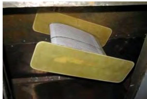
Fig.2.20. Airfoil model with MW-absorbing strip graphite elements on its surface (one can see system of thin parallel dark lines)
