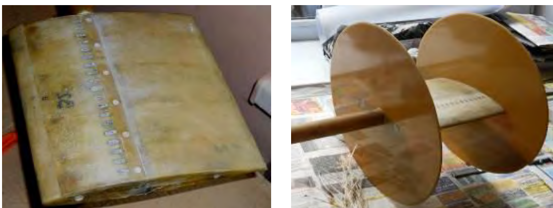
Fig.4.13. New aerodynamic models with ring-type plasma initiators
