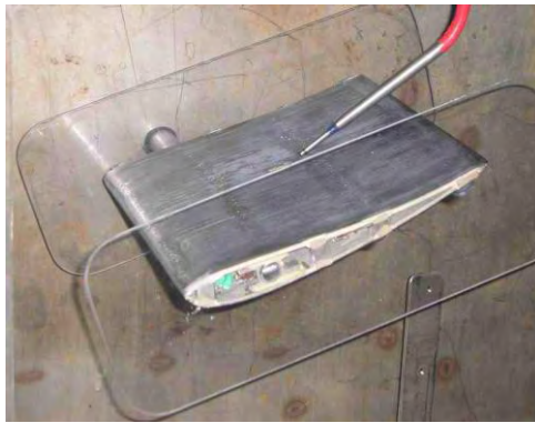
Fig. A7.1. R800 model in the test section with CTA probe holder
