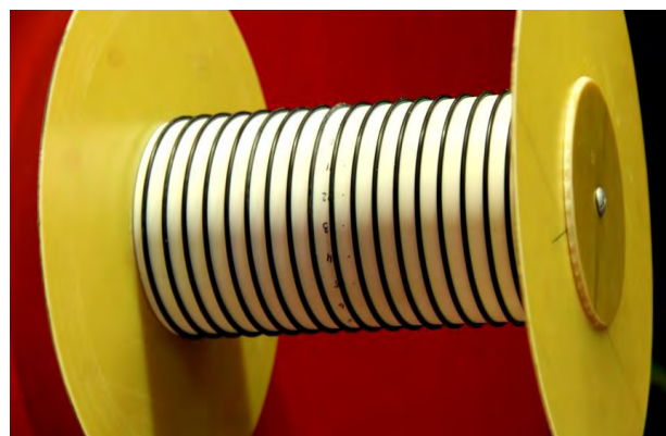
Figure 5.11. Cylindrical model \varnothing 106.6 mm with O-rings, \varnothing 2.5 mm cross-section, \Delta z=10 mm
