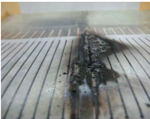
Fig. 7.6. Destroyed surface of model #11_2 because of the non-uniformity of the MW field
