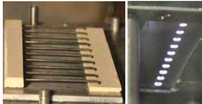
Fig.4.10. External appearance of the vibrator design and system of generated MW discharges
