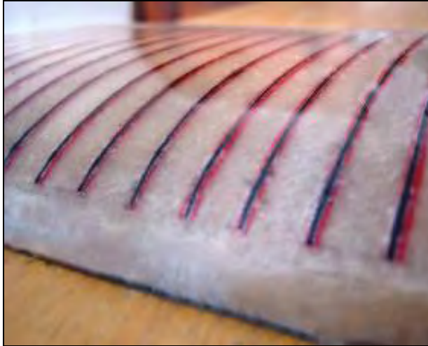
Fig.3.16. Top part of the airfoil model with array of flush mounted MW-heated vibrators
