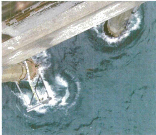
Figure 9. A wave impact event on the instrumented plate. The plate's distance off the pier piling minimizes any flow distortion or wave reflections from the pier piling that the plate is mounted to.
