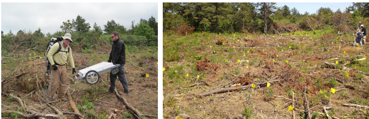
Figure 5-11 – NRL TEMTADS MP 2x2 Cart Deployed in Modified Litter Mode (left) Man-Portable Subarea Surface Clearance Conditions
