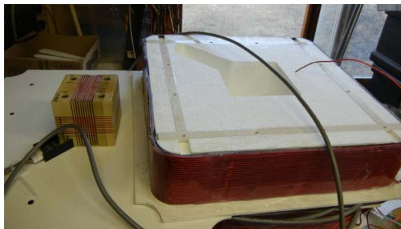
Figure 2-1 – Individual TEMTADS/3D EMI sensor with 3-axis receiver under construction.
