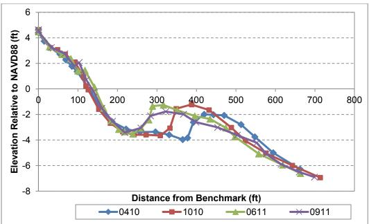
Figure C33. Profile at FMB 32 (including USACE 1009 survey).
