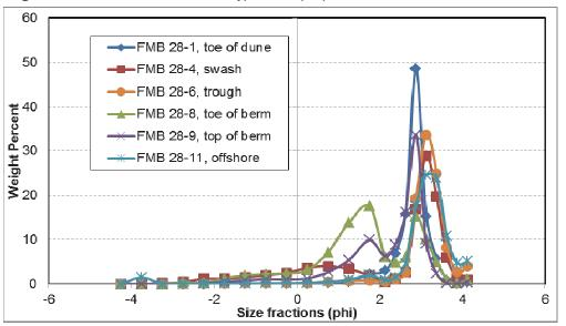
landward terminus of the berm may suggest a landward selective sediment transport of coarser material. The top of the berm was characterized by moderately-sorted fine sand. The sediment along the seaward slope of the berm and offshore was moderately- to well-sorted fine sand. Compared to the southeast control area (Figure 52), the offshore sediment sample contained much less mud.
