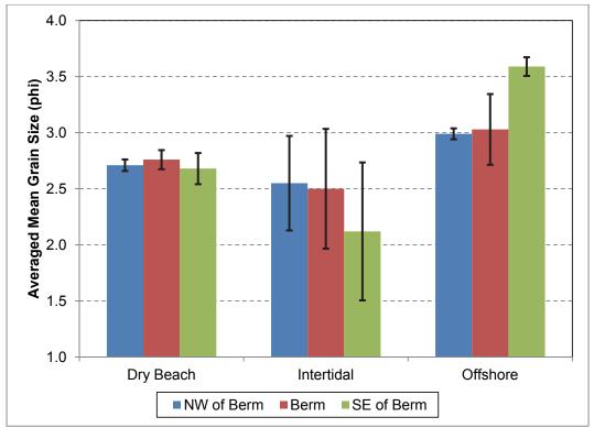
Figure 63. Averaged mean grain size of samples from the dry beach, intertidal zone, and offshore areas southeast of the berm, illustrating spatial and temporal variations in grain size.
