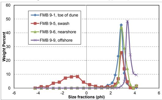
Figure D6. Grain-size distribution at FMB 9 (April 2010).
