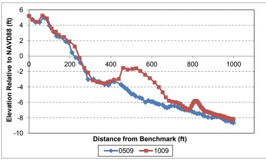
Figure 29. Profile USACE 10 showing constructed berm.
