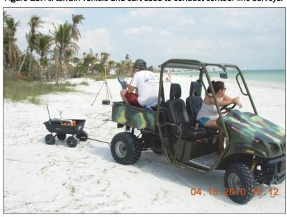
Figure 15. All-terrain vehicle and cart used to conduct contour line surveys.
