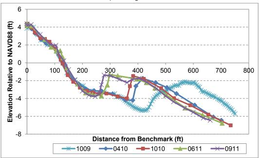
Profiles FMB 43 and FMB 44 represent typical behavior of the profiles at the northwestern section of the berm project. The constructed berm is illustrated by profile USACE 21 (Figure 34). Although the USF-CRL FMB profiles and the USACE profiles do not overlap exactly, here they are within 200 ft of each other. The artificial nearshore berm constructed in this section is relatively narrow as compared to the rest of the berm project,
