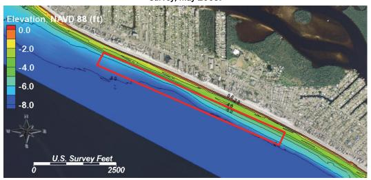
Figure 47. Post-construction bathymetry of berm area (red box) and immediate vicinity, SAJ survey, October 2009.
