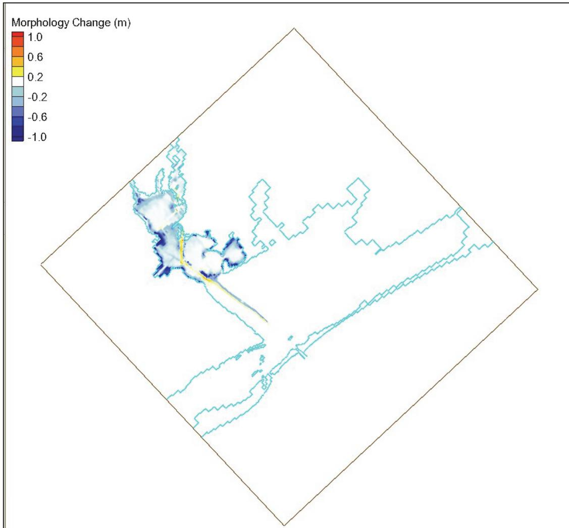
Figure 31. Calculated non-cohesive sediment accretion/erosion, September 2006 to February 2007.
