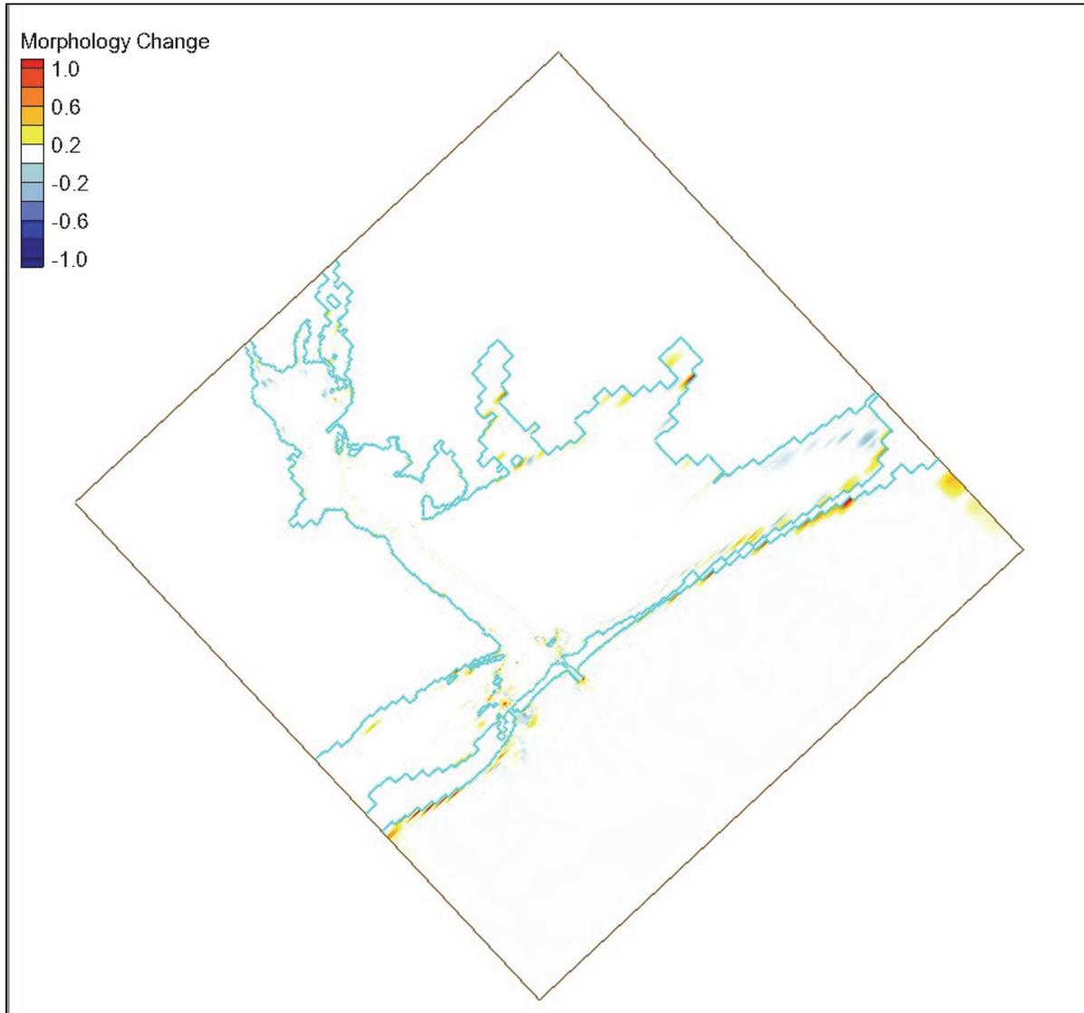
Figure 32. Calculated mixed-sediment accretion/erosion, September 2006 to February 2007.
