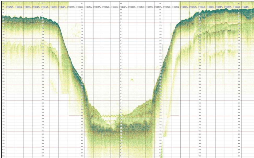
Figure 42. SILAS data analyzed for cross section in the Gulfport Mississippi Ship Channel.
