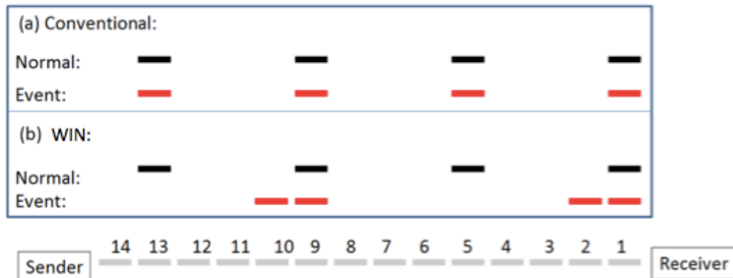
Figure 5. Conventional approach vs. WIN. Time slots labeled by time are shown at the bottom. Solid bars denote normal (black) and event (red) packets transmitted at various time slots.
