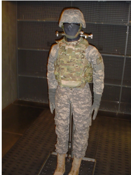
Figure 4. Thermal manikin wearing the female IOTV.
