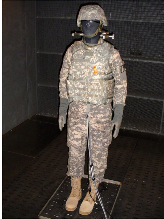
Figure 3. Thermal manikin wearing the IOTV.
