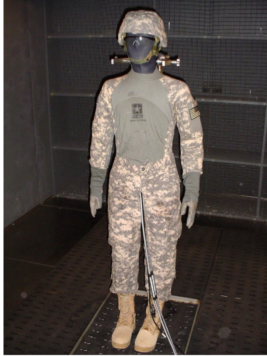
Figure 2. Thermal manikin wearing the Plate Carrier.
