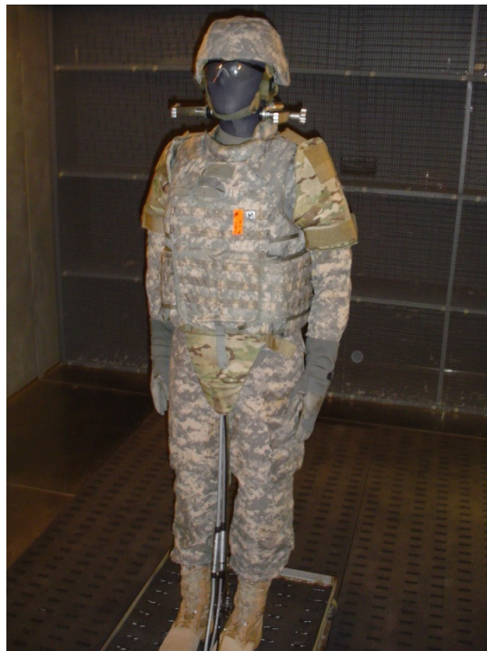
Figure 3. Thermal manikin wearing the IOTV with groin and dorsal protection.
