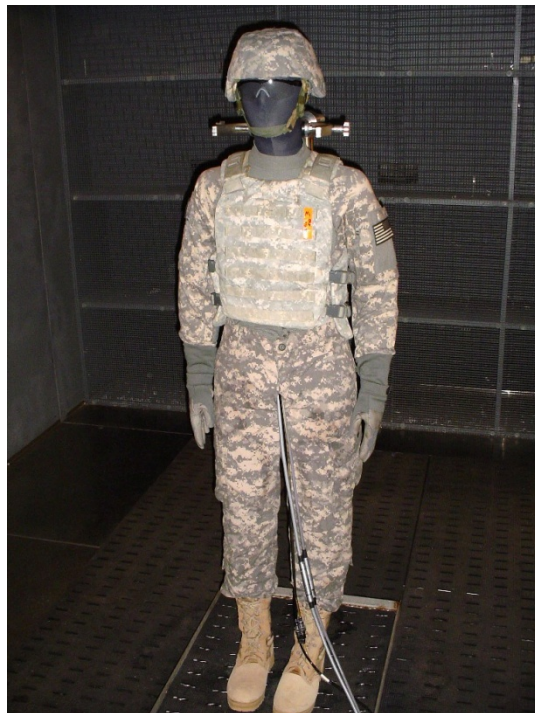
Figure 2. Thermal manikin wearing the Plate Carrier.
