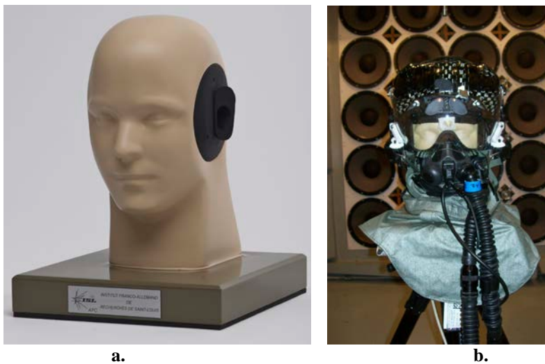
Figure 6. a. Acoustic Test Fixture (ATF) b. ATF in MIRE facility (occluded ear condition)
