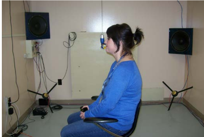
Figure 4. Subject in REAT chamber collecting open ear thresholds
