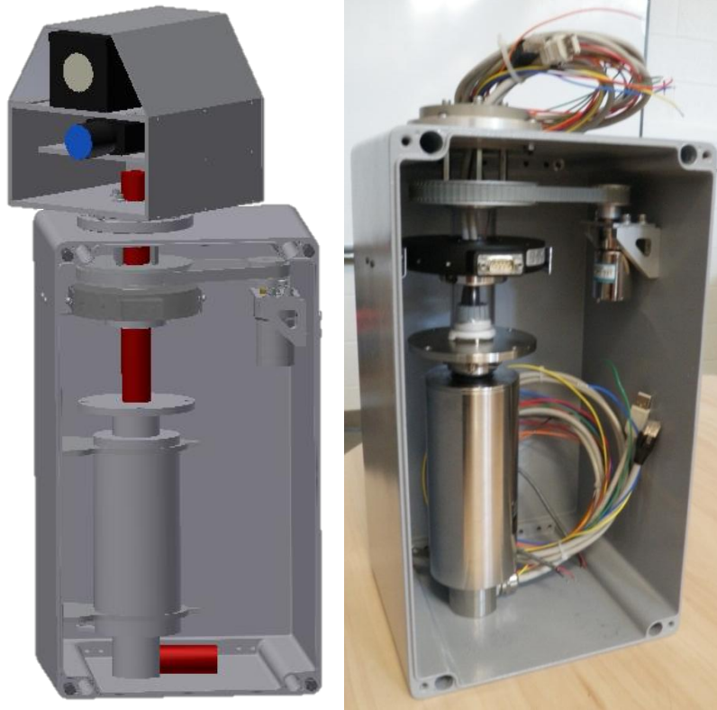
Figure 25. Left: CAD model of the final assembled sensor platform. Right: Current status of the fabricated platform. The slip ring, rotary encoder, belt drive and bearing are assembled. The sensor mount, slip ring mounts and sensors must be added to complete the assembly. Additionally, bulkhead electrical connectors will be added so the enclosure can be sealed.
