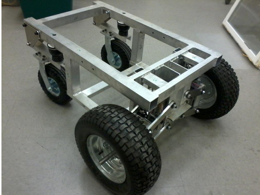
Figure 31. Bare assembled MkIII, Number 1, ready for installation of power and control electronics
