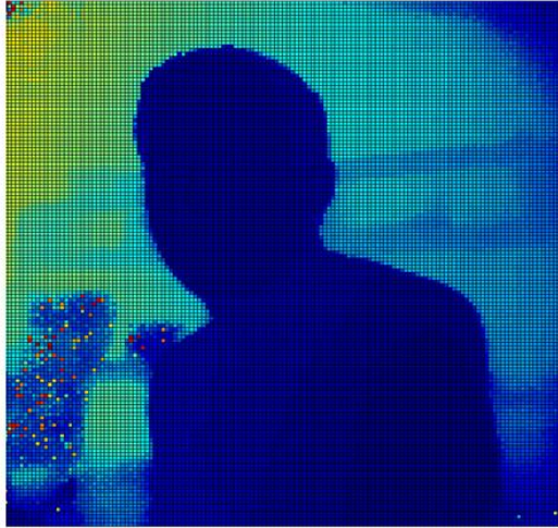
Figure 28. Matlab processed distance data. The left image is a Z-Distance plot in which each pixel is color coded based on the Z-Distance from the sensor. The image on the right is a three-dimensional Cartesian point cloud representation of the same frame.
