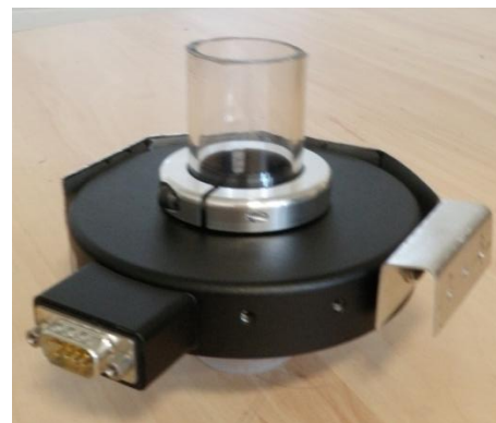
Figure 24. Left: CAD model of the 775 rotary encoder from EPC. Right: Assembled encoder complete with the rotating shaft and a stationary mounting bracket. The shaft inserts into the pulley, which can be observed in the CAD model of Figure 23.
