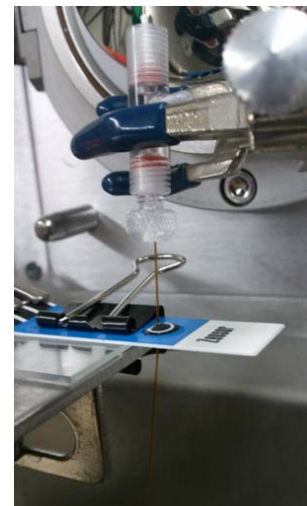
Fig.8: A picture of the nanoDESI setup using the screen printed electrode.
