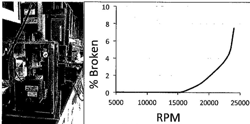
**Figure 3:** (left) Picture of the Couette viscometer with nested cylinders. (right) Plot of percentage of broken microcapsules with a 0.9  $\mu\text{m}$  shell thickness as a function of rotation speed.
