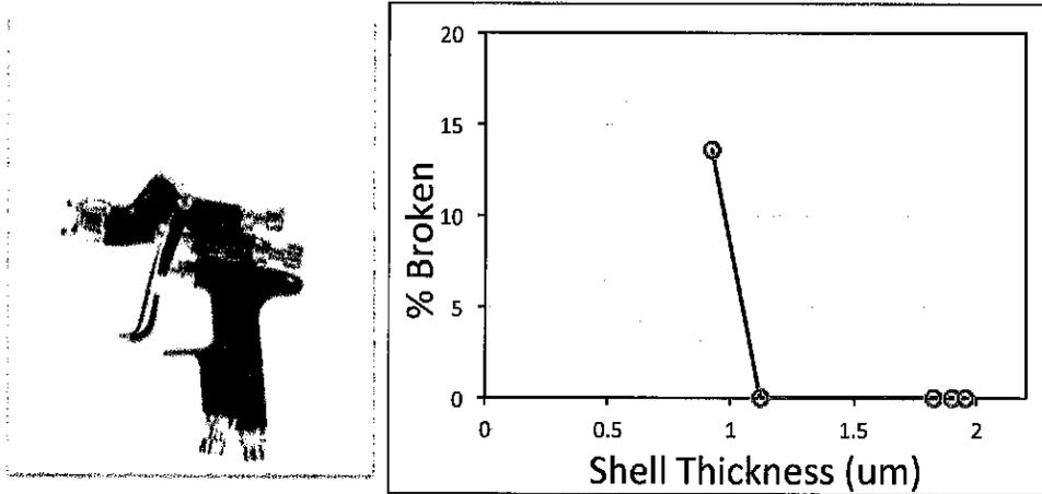
**Figure 2:** (left) HVLV spray gun used for shear experiments. (right) Fraction of broken microcapsules as a function of shell thickness.
