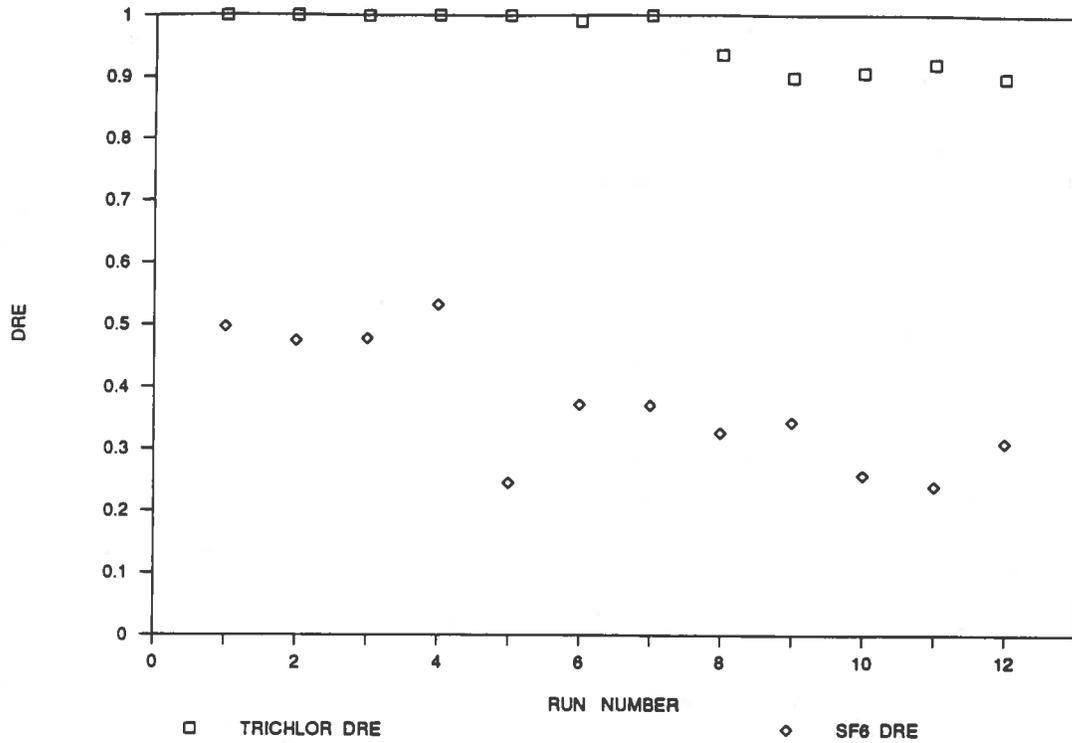
FIGURE 2. Comparison of trichloroethene and sulfur hexafluoride DRE for liquid fuel firing in the incineration tunnel.
