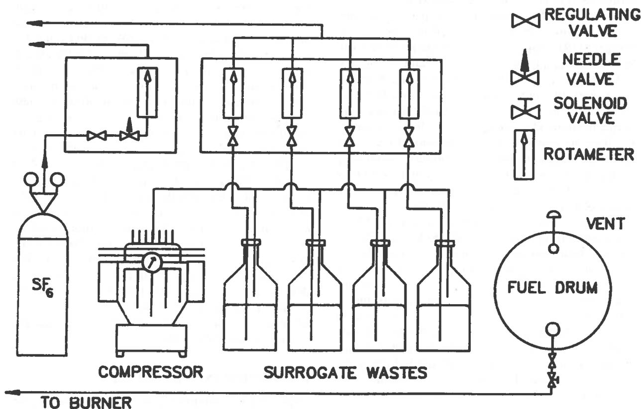
FIGURE 1A. Fuel, waste, and SF<sub>6</sub> injection system.
