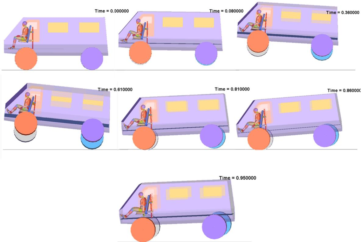
Figure 4.3a Vehicle Kinematics during the entire blast event
