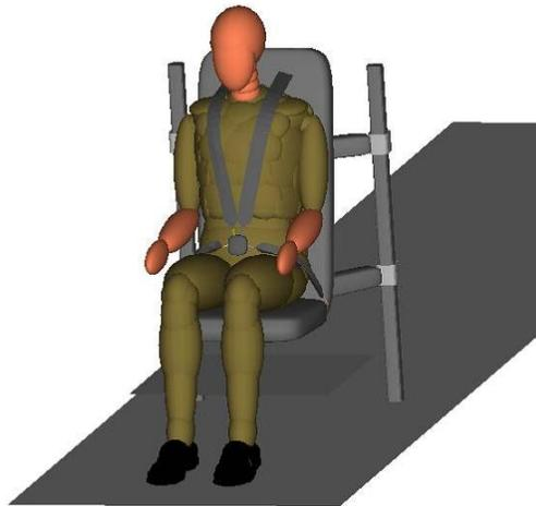
Figure 3.1 Dummy and Harness System Setup
