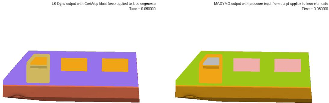
Figure 5.5 LS-Dyna output with ConWep blast force applied to fewer segments, and MADYMO output with pressure from script applied to fewer elements
