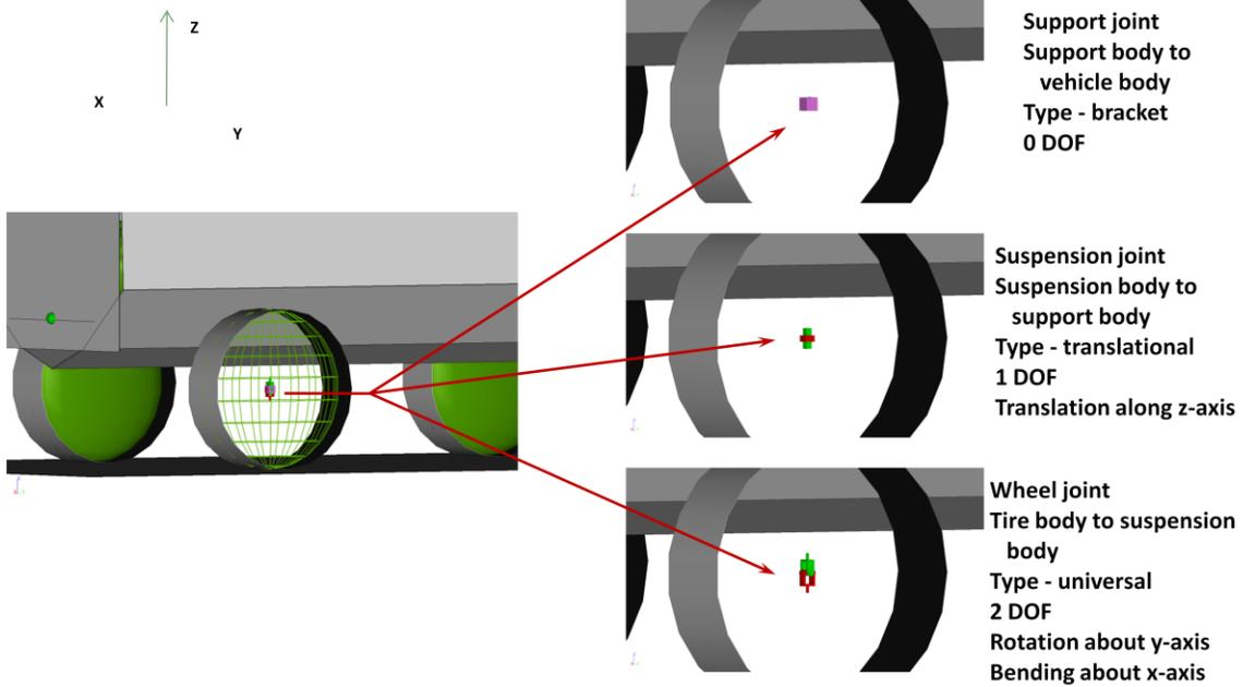
Figure 2.7 Suspension joints
