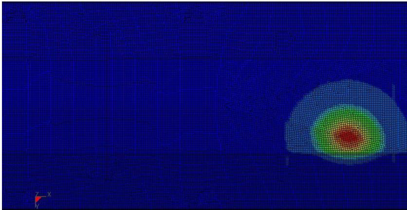
Figure 4.5 Contours of Interface Pressure from Blast
