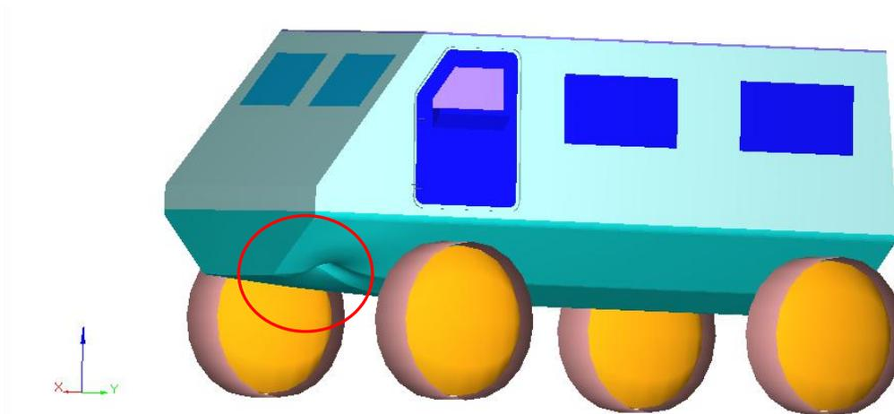
Figure 4.6 Deformation of hull due to blast
