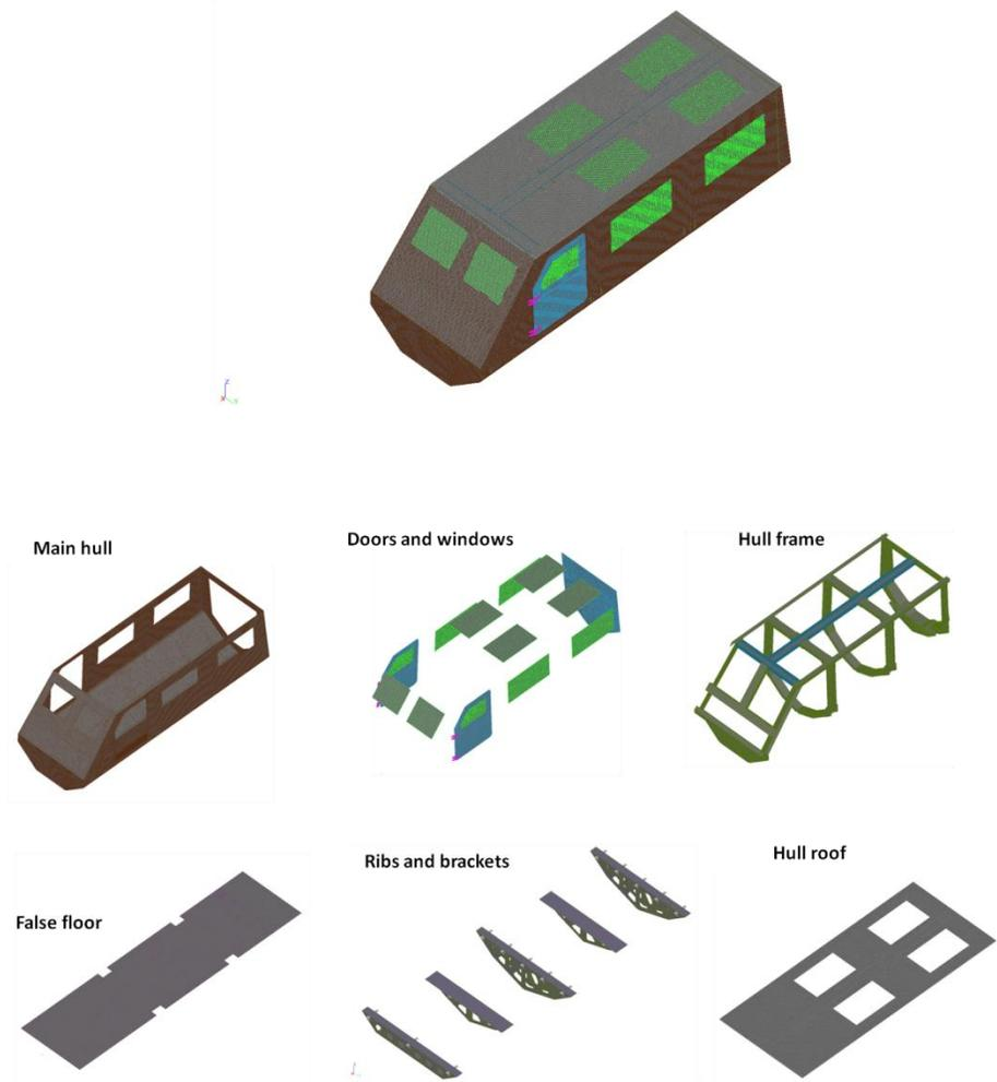
Figure 2.2 Hull full FE model in MADYMO
