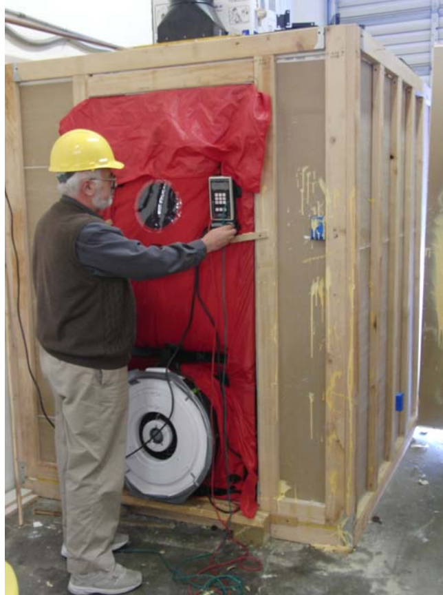
Fig. 9. Testing Shed with Energy Conservatory Blower Door
