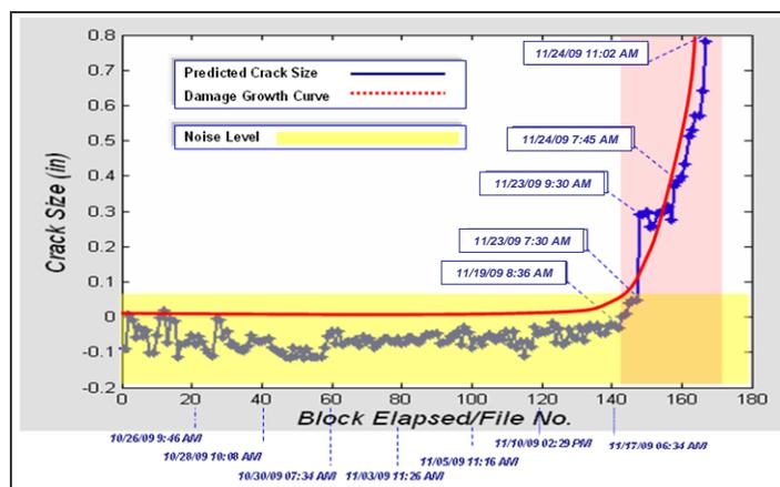
Figure 5: Test Results from Fatigue Crack Monitoring
