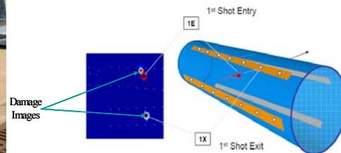
Figure 10: Ballistic Test Result from Damage Detection Imaging
