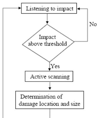
Figure 1: Passive-active System Flow for Damage Detection
