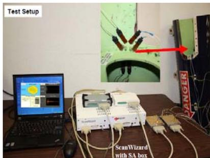
Figure 3: The Test Setup for Fatigue Test
