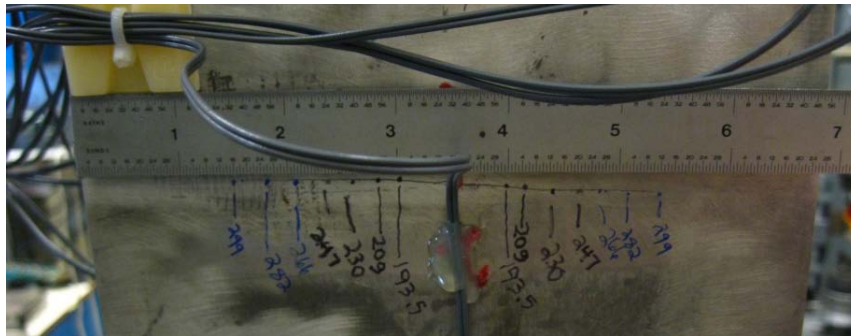
Figure 3. The crack, with propagated length labeled at fatigue cycle counts (in thousands), is visible on the back of the specimen (butt weld covered by ruler).
