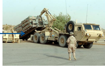
Figure 2: Flatrack carrying "break bulk" load
