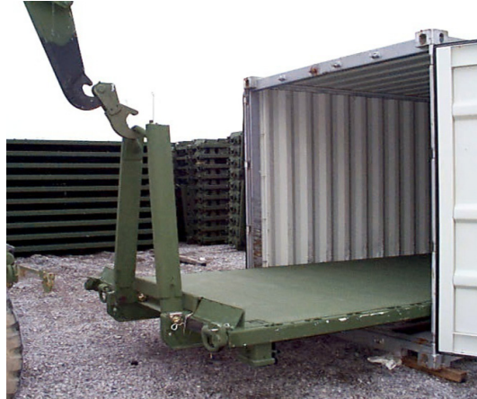
Figure 3: Container Roll-in/out Platform
