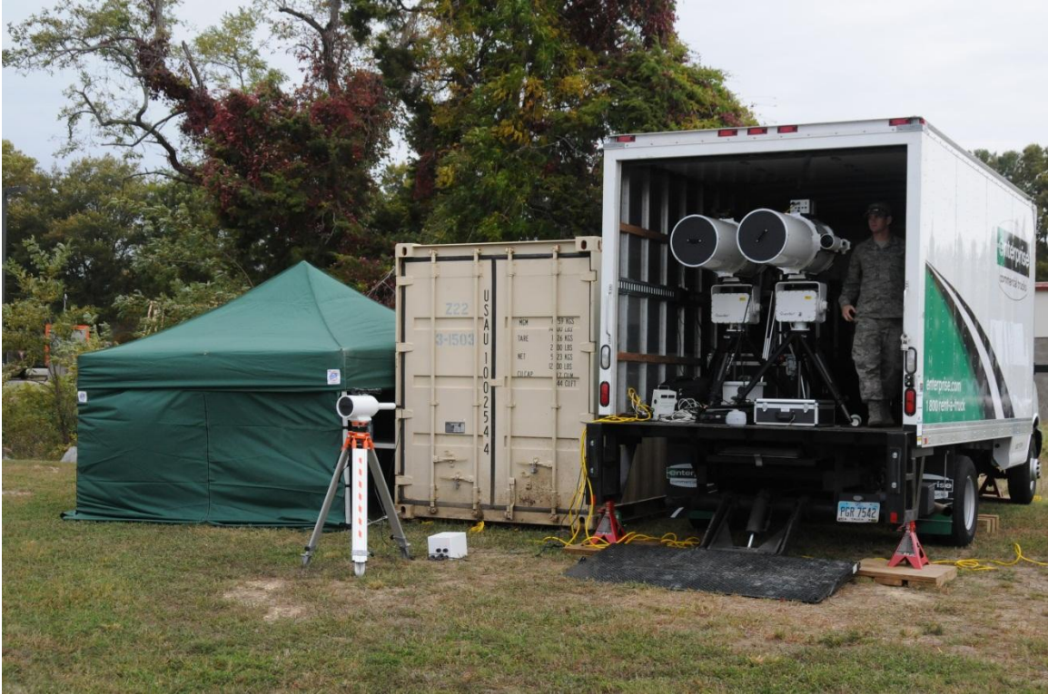
Figure 3b: Picture of the TDLAS main site showing the physical setup of the test equipment at the main test site. The control tent is on the left, the CONEX storage container is in the middle, and the box truck containing the majority of the test equipment is on the right. The BLS 900 Scintillometer receiver and processing unit are located in front of the CONEX.
