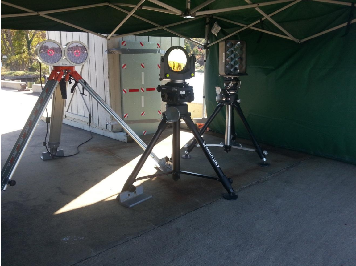
Figure 4b: A picture of the mirror site showing the physical layout of the test equipment. On the left is the BLS 900 Scintillometer transmitter, in the center is the 6" turning mirror, and on the right is a crude retro reflector array borrowed from Dahlgren NSWC. A large foam rectangle with reflective strips was taped to the shed behind the test equipment to aid in alignment.
