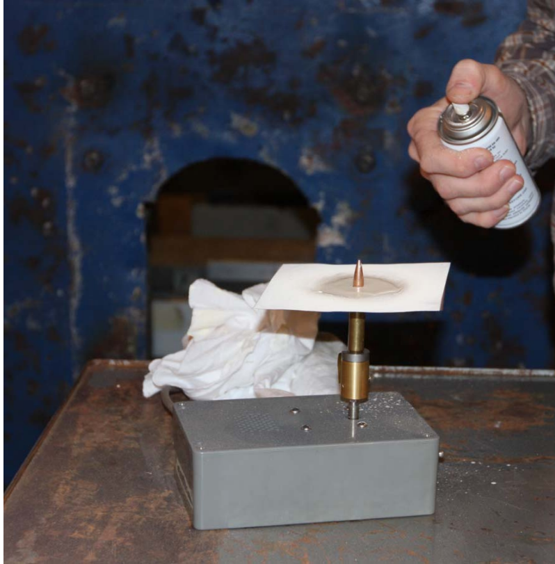
Figure 4. Rotating device for coating ammunition with HBN.
