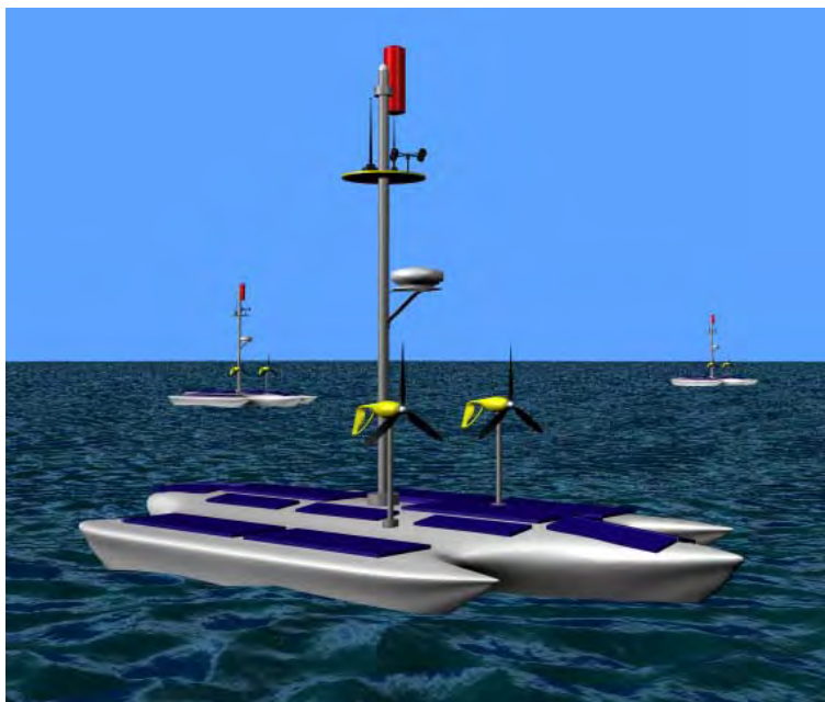
Figure 2.3: The ASC Sea Rover concept vehicle depicts a UMS designed specially for ATON missions. Many operational concepts involve the augmentation of traditionally moored buoys with “smart” UMS buoys that could send navigation information as well as receive and relay maritime domain awareness information. From [6].
