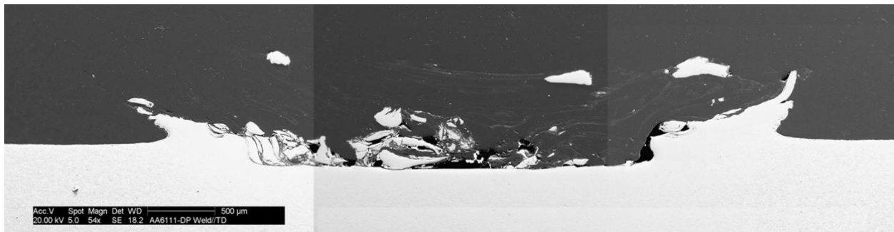
Figure 14 Composite of SEM micrographs at 100x magnification, showing weld cross section and turbulent WZ structures.
