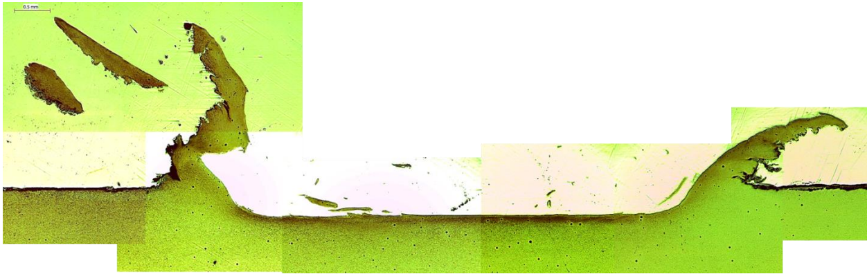
Figure 32 Composite of optical micrographs at 10x magnification showing weld cross section.
