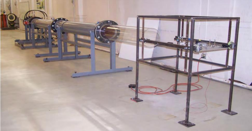
Figure 1. WSU Bioengineering Center Shock Tube.
