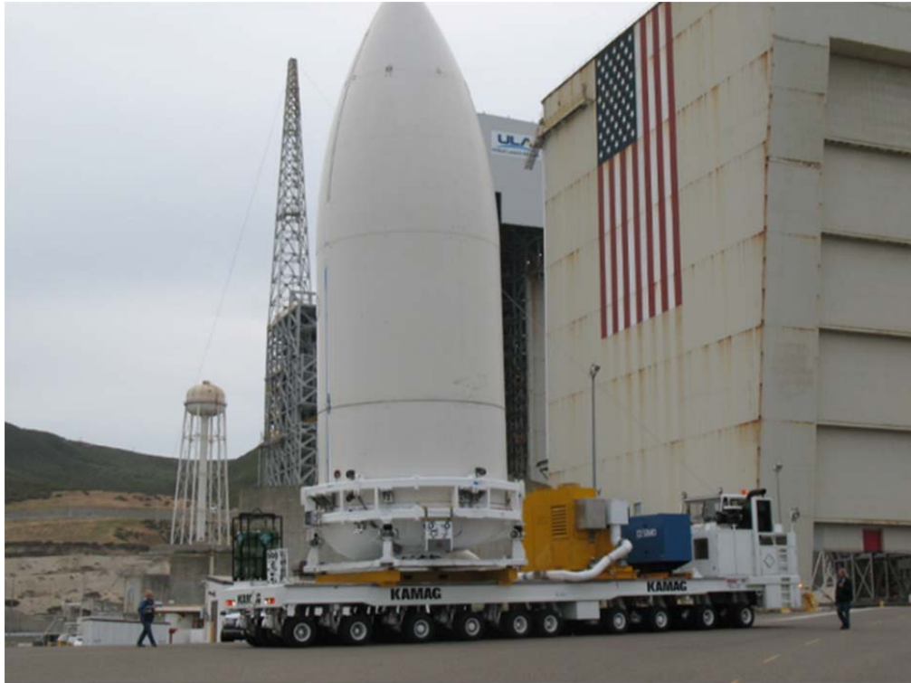
Figure 14. KAMAG with Encapsulated Assembly
