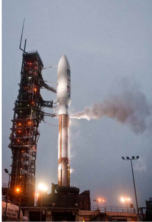
Figure 34. Cryogenic Tanking Prior to Launch
