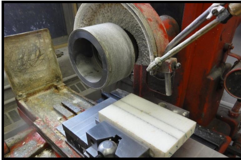
Figure 6. Blocks reduced to a thickness of 2.54 cm using surface grinder and custom electroplated diamond coated wheels
