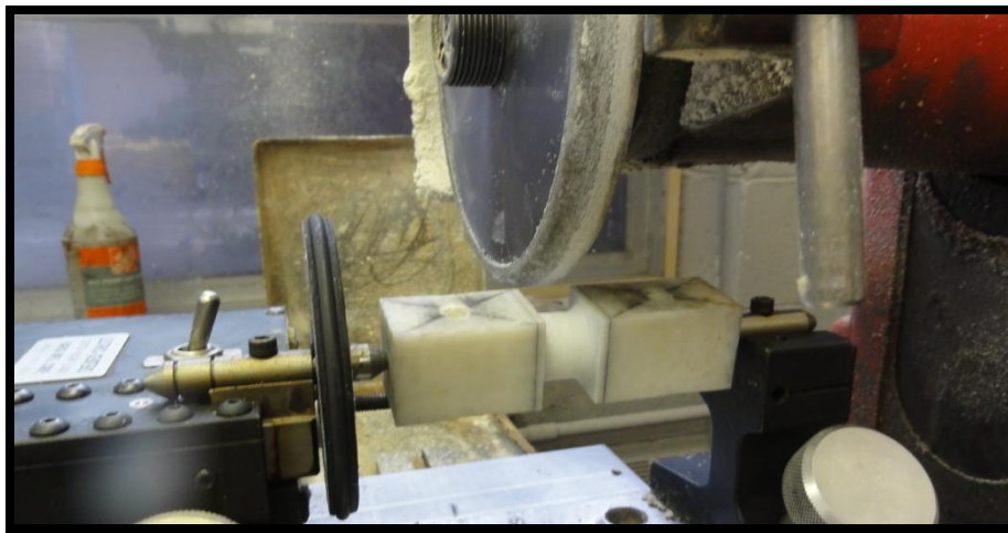
Figure 9. Spooling of out-of-plane tension specimens
