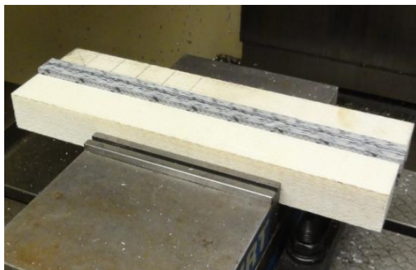
Figure 5. Bonded block in CNC mill prior to (a) and after (b) squaring all sides
