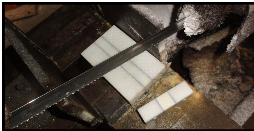
Figure 7. Composites saw cut into 2.54 cm thick by 2.67 cm wide blocks
