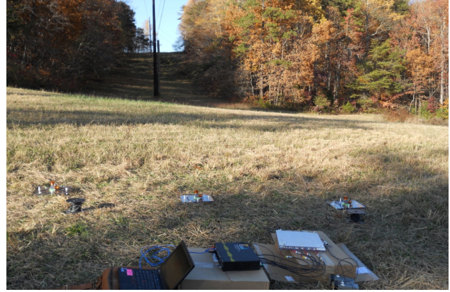
Figure 4b. Three Sensor Pairs and Data Acquisition System Under 69 kV Transmission Line
