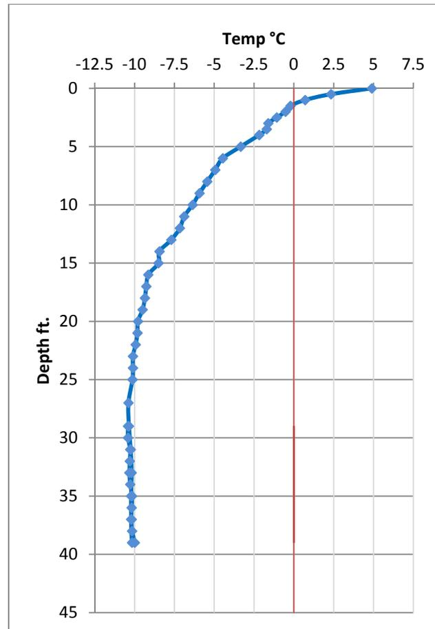
Figure 4. Plot of undisturbed permafrost temperature down to 40 ft below the surface. The depth of zero annual amplitude is approximately at 25 ft where the permafrost is approximately  $-10.0^{\circ}\text{C}$ .
