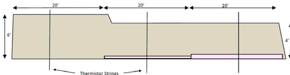
Figure 24. Cross-section of the insulation test embankment.
