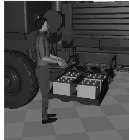
Figure 6. Depiction of battery tray at carrying height.
