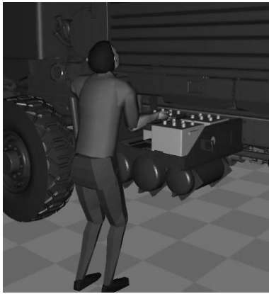
Figure 3. Posture used to lift rear battery.
