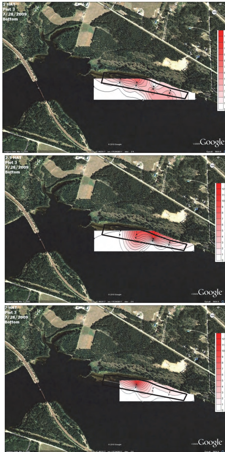
Figure 11. Dye dissipation pattern ( \mu\text{g/L} ) at bottom depth zone, Plot 3 (dye + herbicide treatment) at 1, 2.5, and 7 hr after treatment, Noxon Rapids Reservoir, Montana, 28 July 2009.
