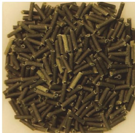
Figure 1. M1 propellant manufactured as extruded tubes.
