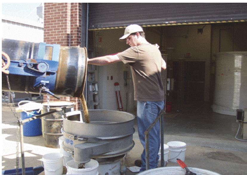
Figure 2. Sieving soil through a ¼-inch mesh screen using a Sweco® Vibro-Energy® Separator.
