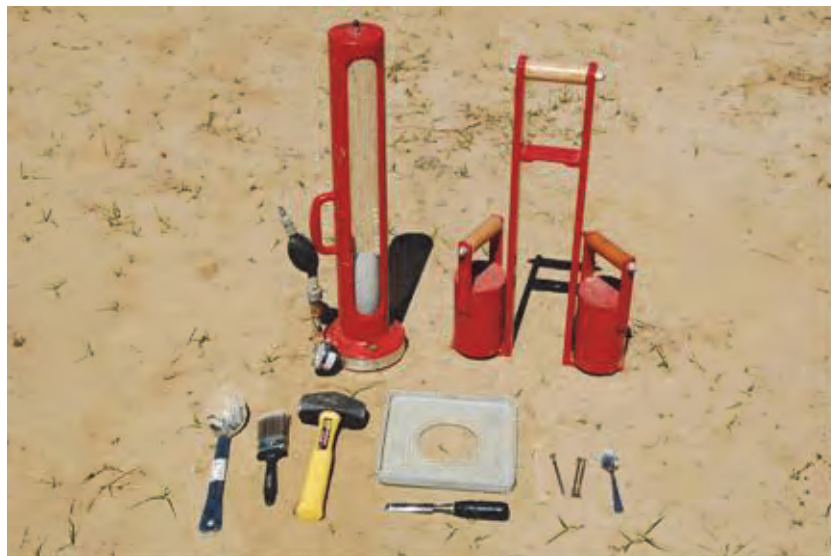
Figure 13. Humboldt Voluvessel (water balloon) and hanging weights.
