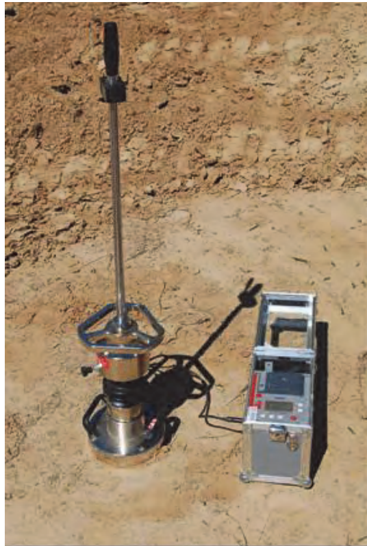
Figure 8. Zorn Lightweight Deflectometer with attached data logger.
