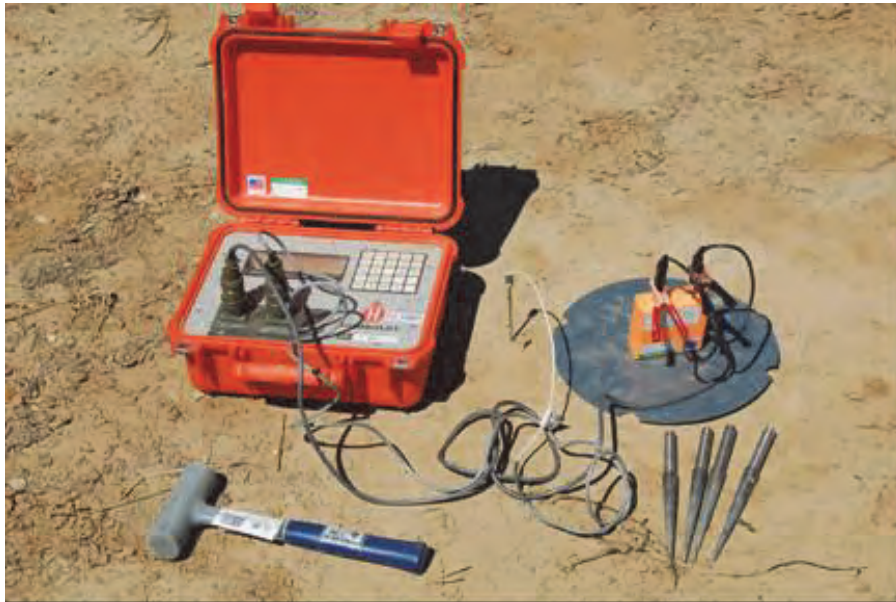
Figure 3. Electrical Density Gauge (EDG), Model H-4114C.3F.
