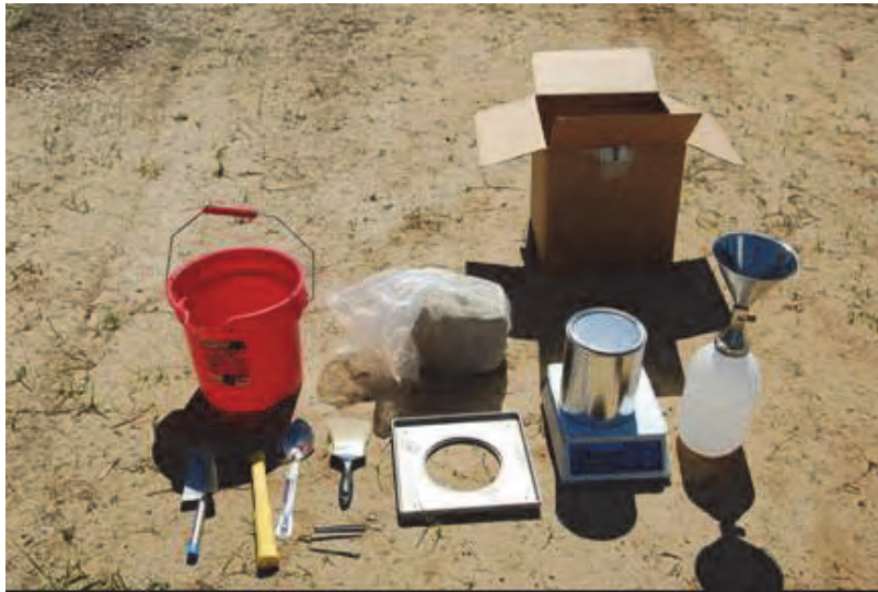
Figure 11. Sand Cone Density apparatus and accessories.
