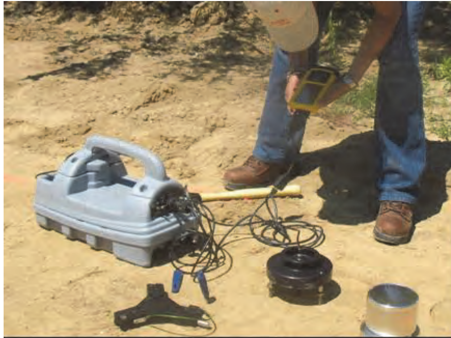
Figure 2. Moisture-density Indicator (M + DI) MDI-2000. Handheld PDA used for data collection.
