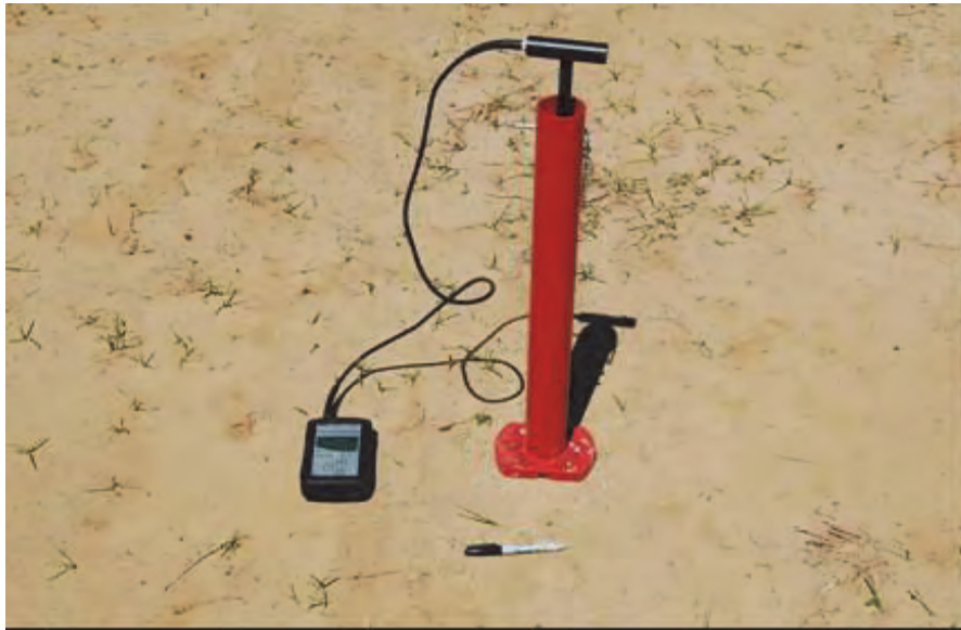
Figure 9. Clegg Hammer with attached data logger.
