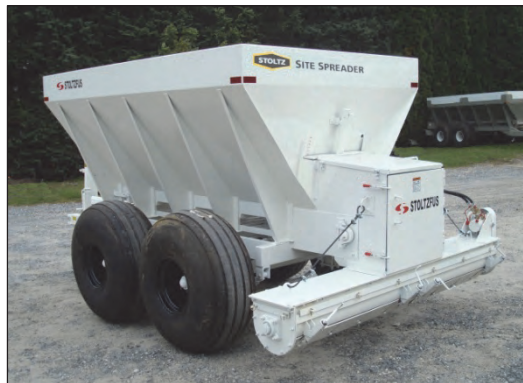
Figure C4. Tractor pulled cement spreader: Designed by Stoltz.
