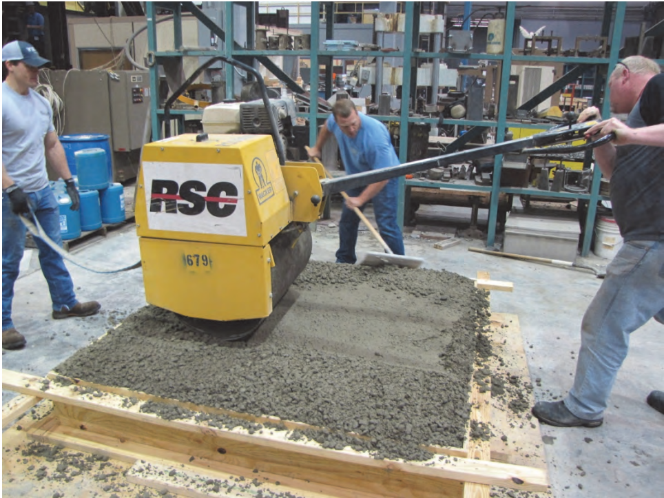
Figure B6. Second lift of concrete being roller compacted.
