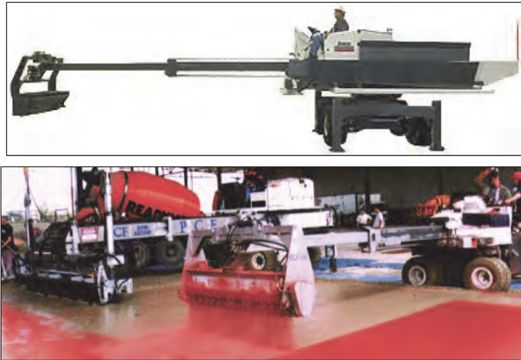
Figure C3. Mechanically operated spreader: Designed by Somero (Model STS-132 Somero Spreader).
