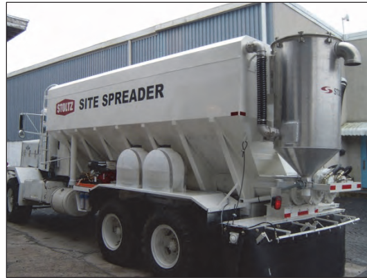
Figure C5. Operated vehicle cement spreader: Designed by Stoltz.
