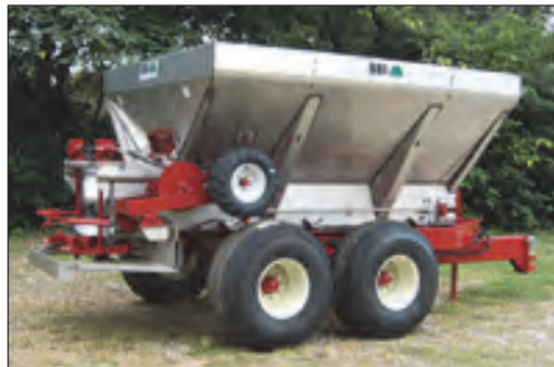
Figure C8. Tractor-pulled lime/fertilizer spreader: Designed by Liberty Mechanical (Model Power Fertilizer Lime Spreader 00LTY).
