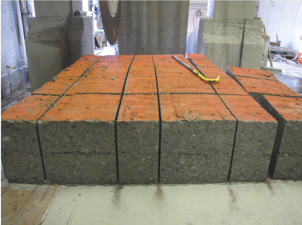
Figure B10. Test slab being cut into specimens for shear testing and coring.
