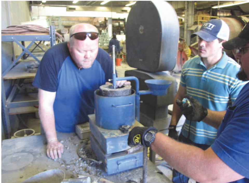
Figure B1. Vebe test being conducted prior to concrete placement.
