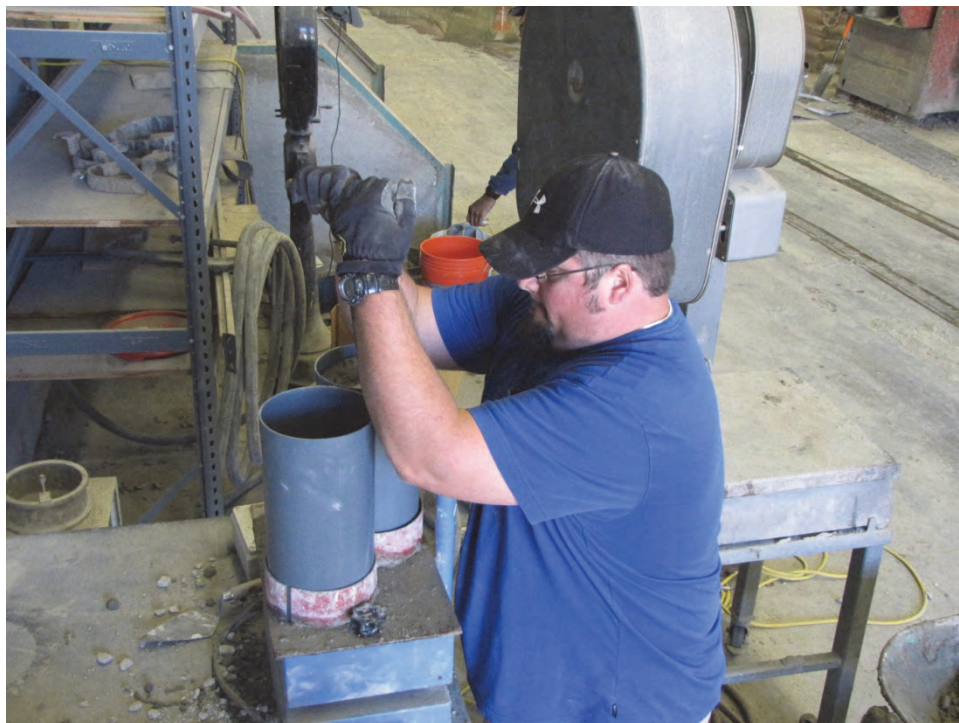
Figure B8. Cylinder being cast using the Vebe vibrating table.
