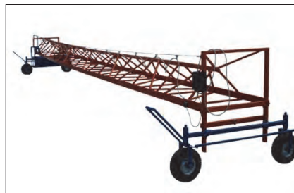
Figure C2. Manually pushed spreader bridge: Model designed by Alexey Gerasimchuck.
