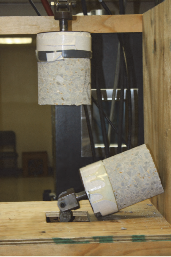
Figure B13. Concrete core after tension test was completed.
