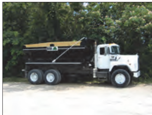
Figure C9. Truck-mounted aggregate spreader: Designed by BBI (Model RockBody 00RB).
