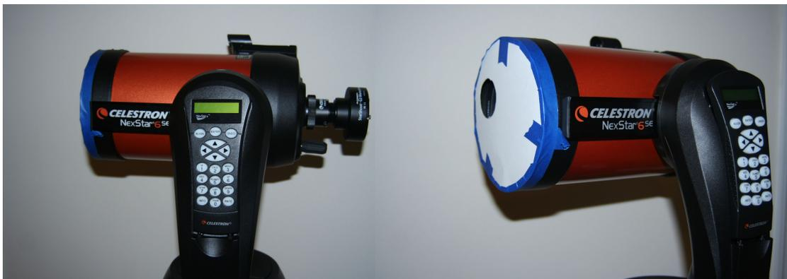
Figure 2.3: Experimental sensor setup consists of a Celestron® NexStar® 6SE 1.5 m focal length telescope with a mask to reduce the aperture to 5 cm, and an Orion® Starshoot™ G3 monochrome camera.
