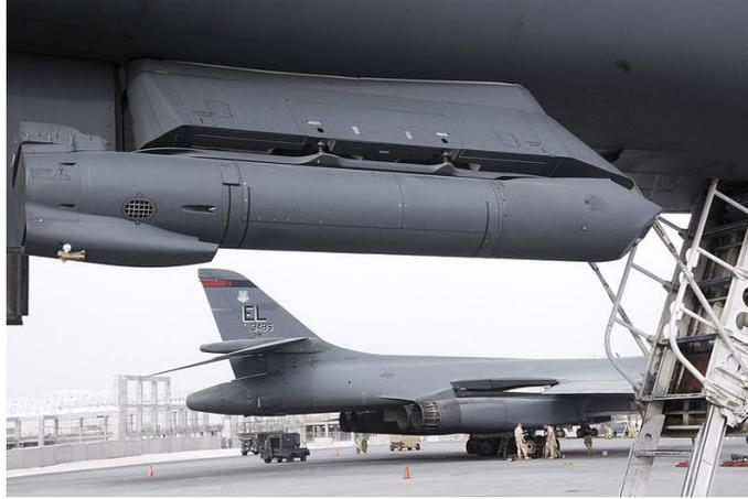
**Figure 1.1: AN/AAQ 33 - SNIPER targeting pod integrated onto the B-1B.**
