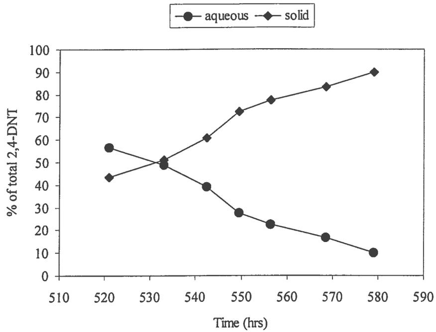
Figure 56 Partitioning in Reactor C at 5% solids loading rate of BAAP soil: Percentage of aqueous phase vs. solid phase 2,4-DNT
