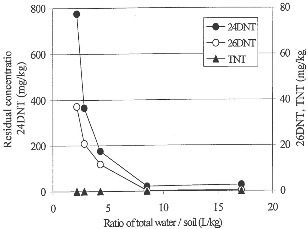
Figure 12 Effects of water/soil ratio on soil washing efficiency: Residual concentration in BAAP soil
