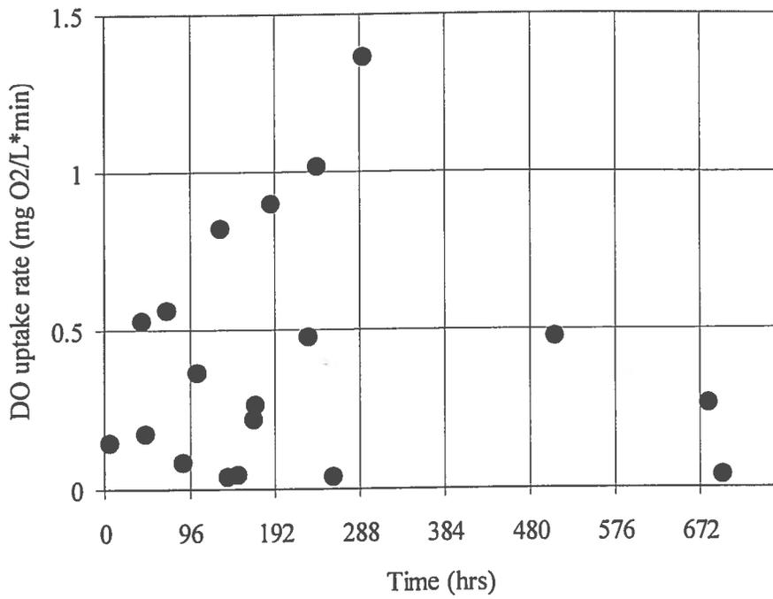
Figure 24 Oxygen uptake rate in Reactor A
