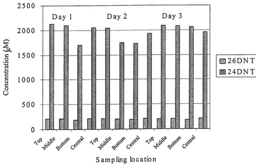
Figure 5 Aqueous phase contaminant concentration profile: BAAP soil at 10% solids loading rate
