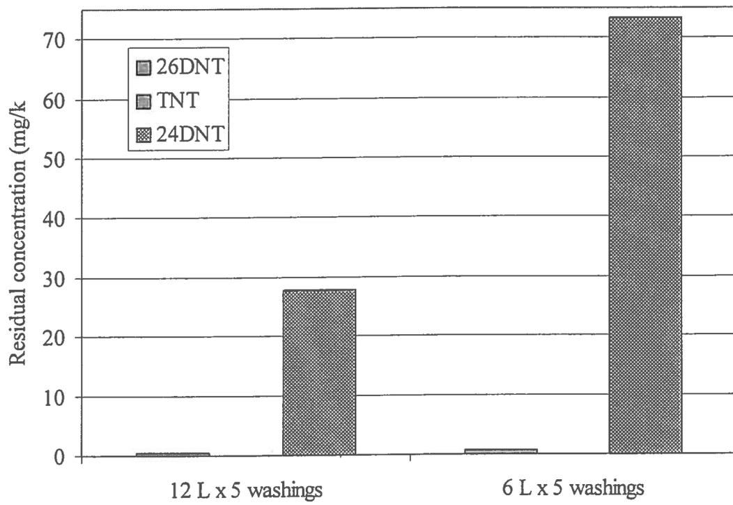
Figure 9 Soil washing efficiency based on residual concentration (BAAP soil): 12 L x 5 washings vs. 6 L x 5 washings
