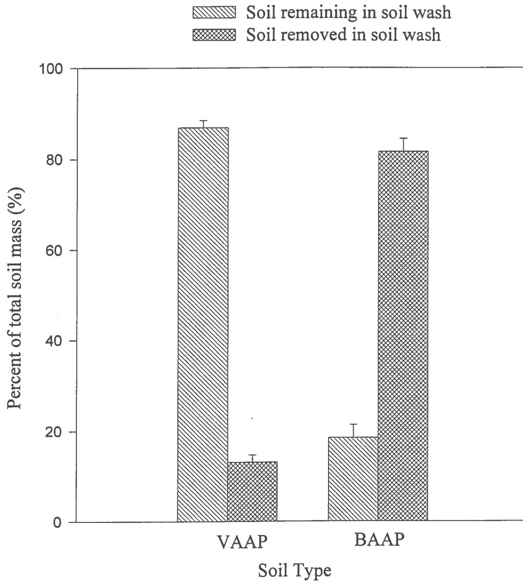
Figure 8 Soil mass distribution after soil washing
