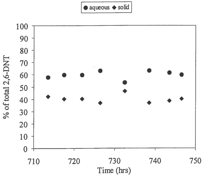
Figure 59 Partitioning in Reactor C at 10% solids loading rate of BAAP soil: Percentage of aqueous phase vs. solid phase 2,6-DNT
