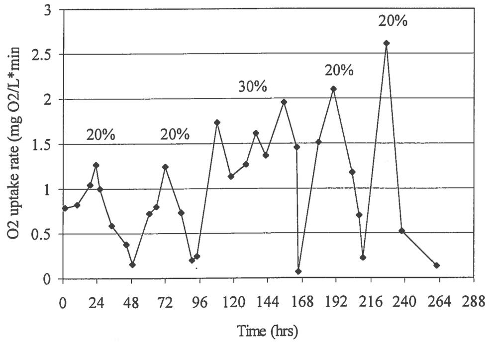
Figure 44 Oxygen uptake rate in Reactor E
