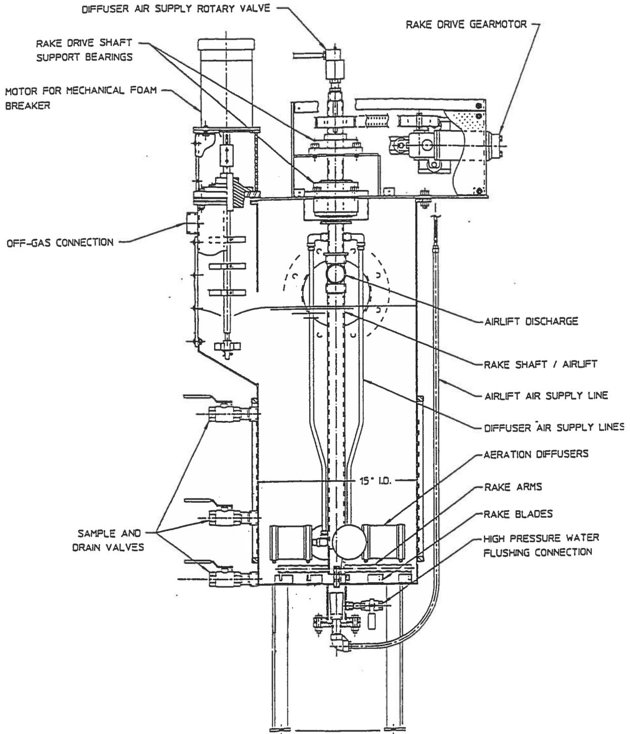
Figure 1 Schematic of Eimco Biolift Slurry Reactor
