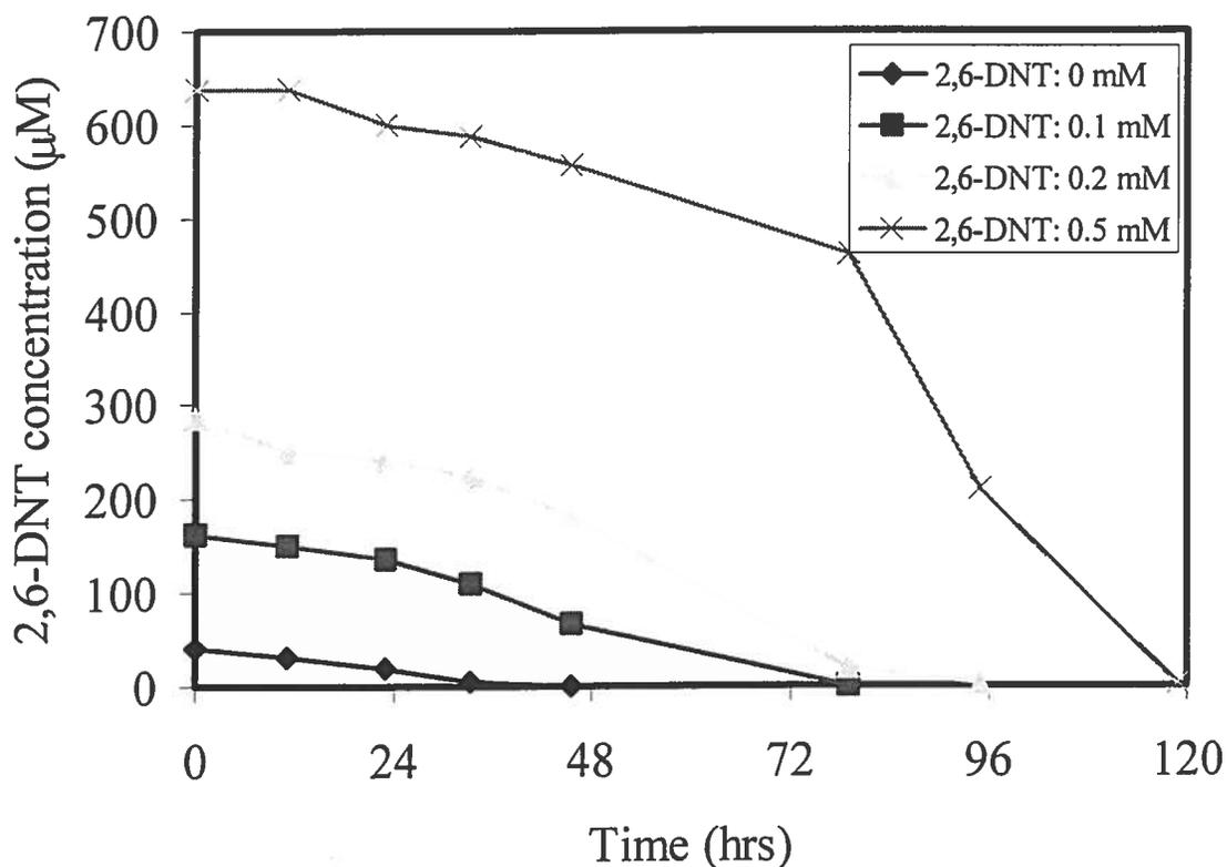
Figure 71 Degradation of 2,6-DNT at various initial concentrations
