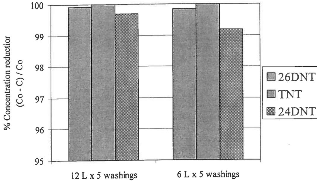
Figure 10 Soil washing efficiency based on concentration reduction (BAAP soil): 12 L x 5 washings vs. 6 L x 5 washings
