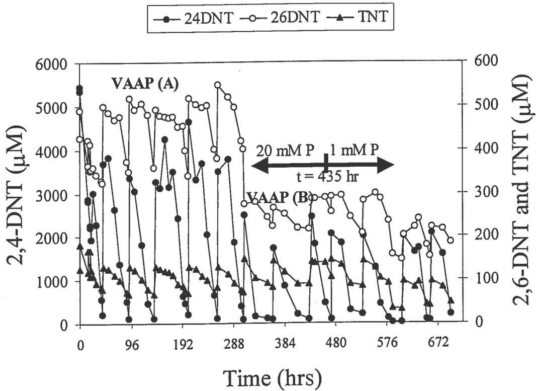
Figure 20 Degradation of 2,4-DNT, 2,6-DNT and TNT in Reactor A
