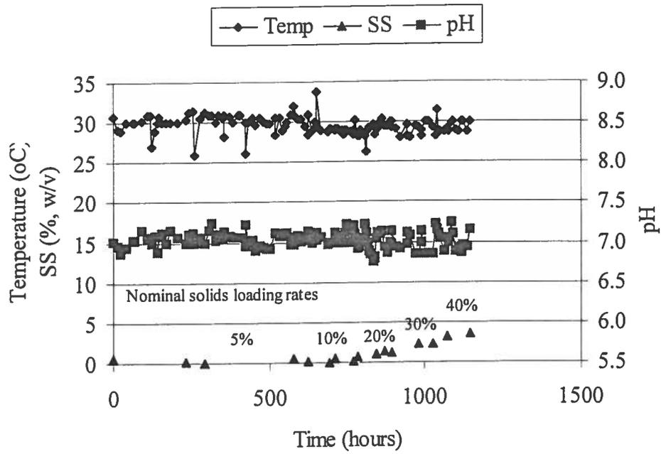
Figure 28 Variation of temperature, pH and SS in Reactor C
