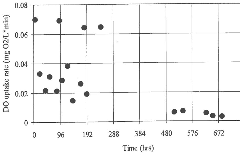
Figure 25 Oxygen uptake rate in Reactor B
