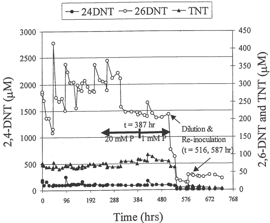
Figure 21 Degradation of 2,4-DNT, 2,6-DNT and TNT in Reactor B
