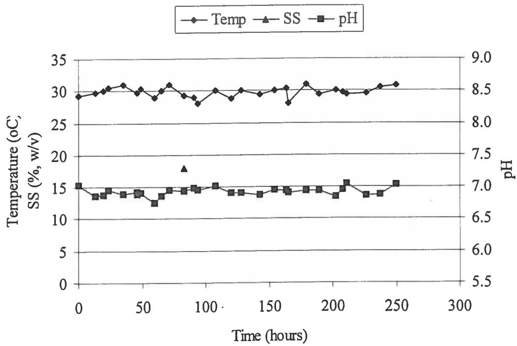
Figure 39 Variation of temperature, pH and SS in Reactor E
