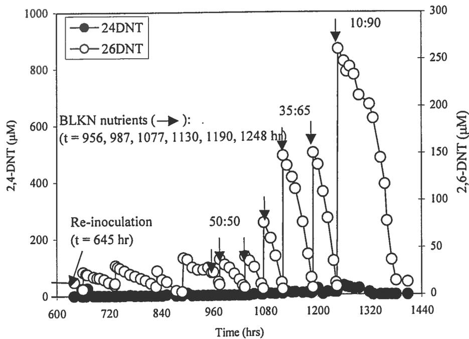
Figure 32 Degradation of 2,4-DNT and 2,6-DNT in Reactor D: Fill-and-draw mode with effluent from Reactor C
