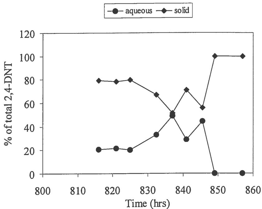
Figure 60 Partitioning in Reactor C at 20% solids loading rate of BAAP soil: Percentage of aqueous phase vs. solid phase 2,4-DNT
