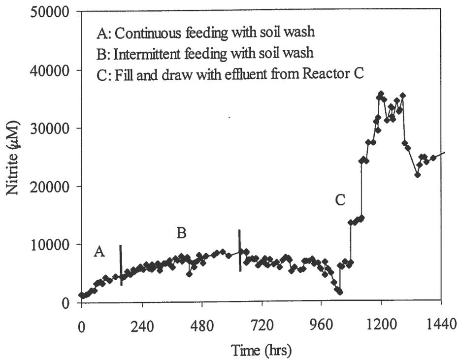
Figure 34 Nitrite concentration in Reactor D
