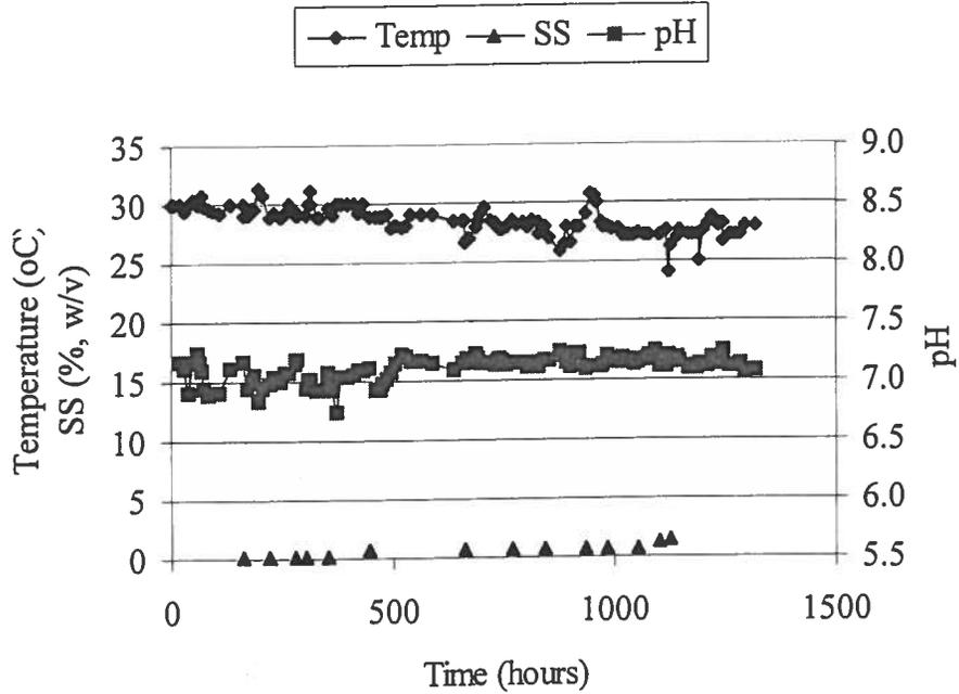
Figure 29 Variation of temperature, pH and SS in Reactor D
