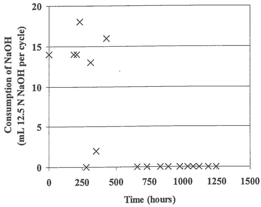
Figure 38 NaOH consumption in Reactor D
