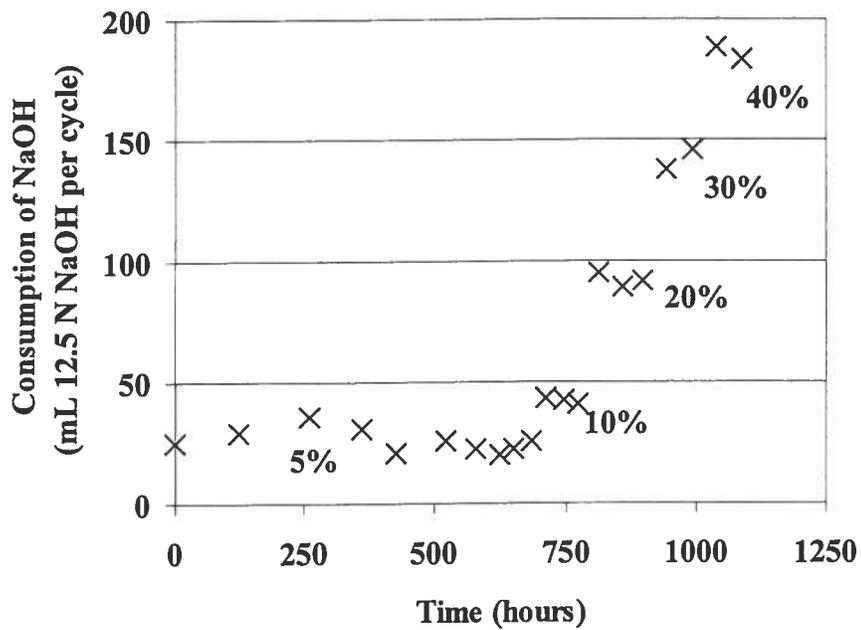
Figure 37 NaOH consumption in Reactor C
