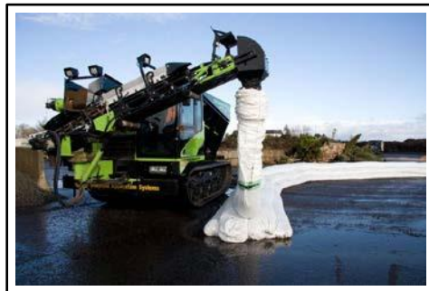
Figure 15. CAS tracked loader (TR30) for geotextile tubes.
