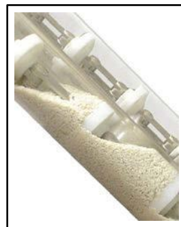
Figure 17. Tubular drag conveyor.
