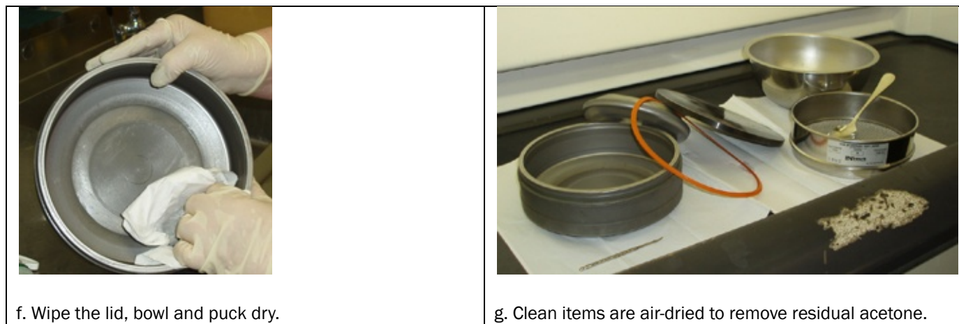
Figure 8.2 How to process a soil sample.
