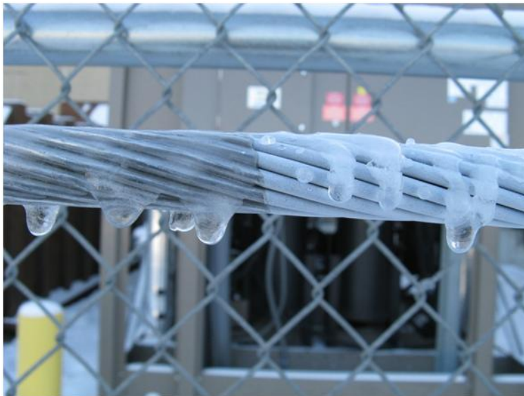
Figure B-5. ETL coated with ISurTec coating right, with bare aluminum surface on left.
