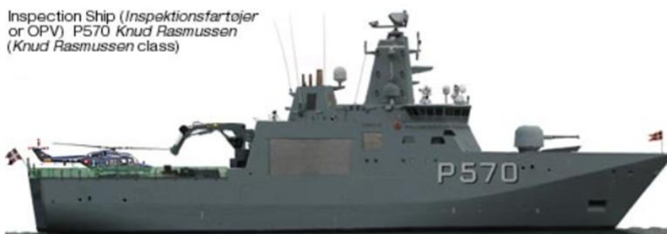
Figure 5-20. Danish Knud Rasmussen -Class inspection ship with enclosed starboard small boat stowage and launch facilities to minimize superstructure icing effects. (image courtesy Stephen Priestley—Canadian American Strategic Review www.casr.ca/ ).
