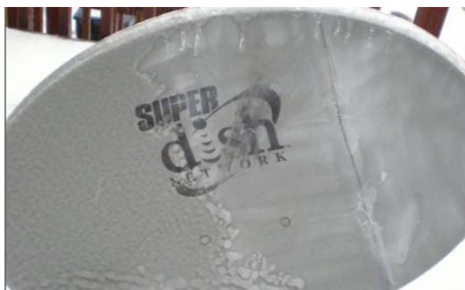
Figure B-15. Ice-free NeverWet SE coated surface (right), and ice-covered uncoated surface (left), of satellite dish after freezing rain storm (Image courtesy Ross Technologies).
