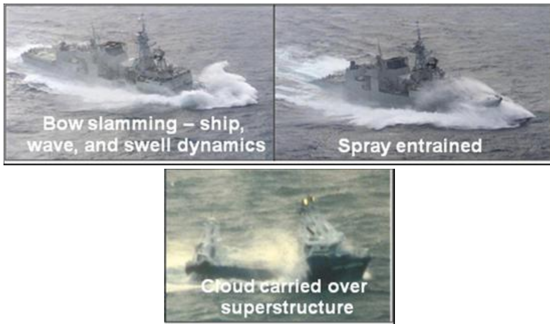
Figure 3-1. Icing modes. Upper left—lofting—bow of Canadian Frigate HMS Fredricton plunging into swell and lofting water jet. Upper right—entrainment—spray is entrained in relative wind and is carried as a pulse of water over the forecastle and is impinging the bridge (upper photos courtesy of http://www.navy.forces.gc.ca/fredricton/0/0-s_eng.asp ). Lower image—traverse—fishing trawler in Bering Sea with spray cloud pulse mid-ships (Ryerson 1990).
