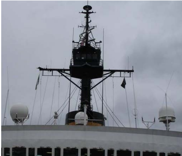
Figure 4-14. Satellite deck electronic equipment is rarely impacted by icing, but is affected by cold (CRREL 2012).
