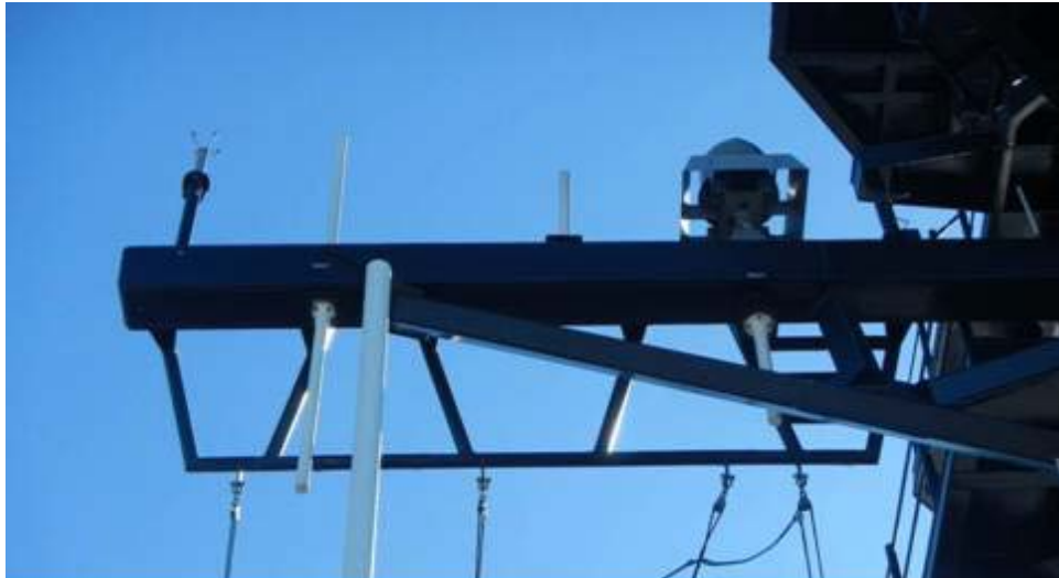
Figure 4-50. Starboard mast upper cross arm with anemometer (left), and various dipole and other antennas (Ryerson 2012).
