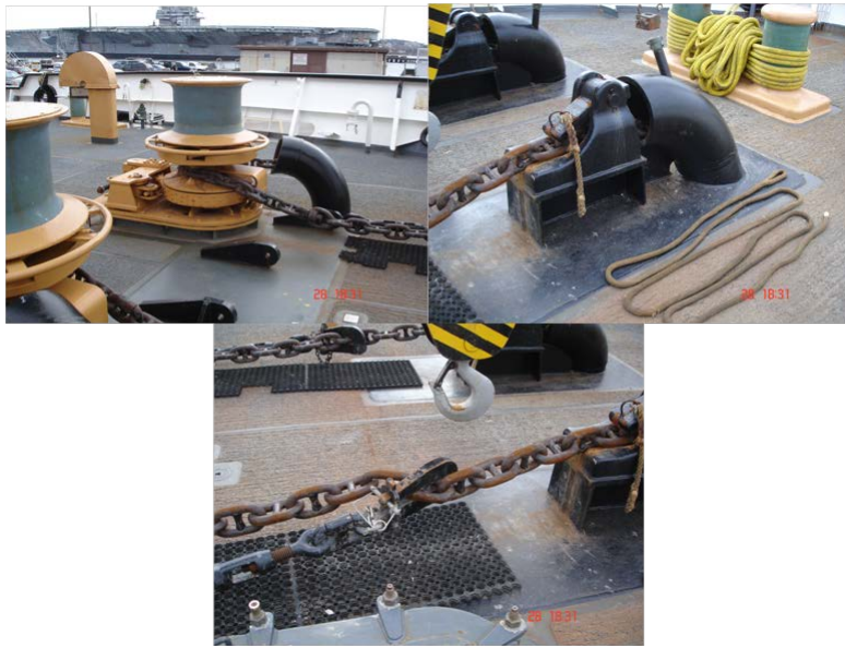
Figure 4-72. Wildcat (upper left), catspaw (upper right) and pelican hook (bottom) require de-icing before releasing anchor (Ryerson 2012).
