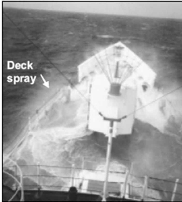
Figure 3-3. Water flowing from flooded forecastle on CGC MIDGETT and drops being entrained in wind after bow spray event in Bering Sea (Ryerson 1990).
