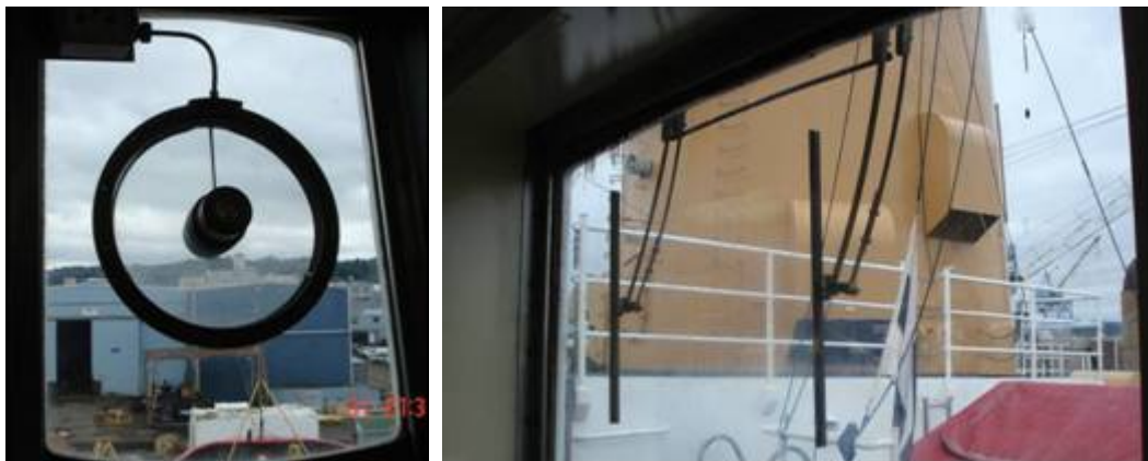
Figure 4-13. Effective Clearview heated spinning window on Left. Right—complex external wiper mechanism that keeps blades parallel to window edge during stroke, but accumulates ice and freezes (CRREL 2012).
