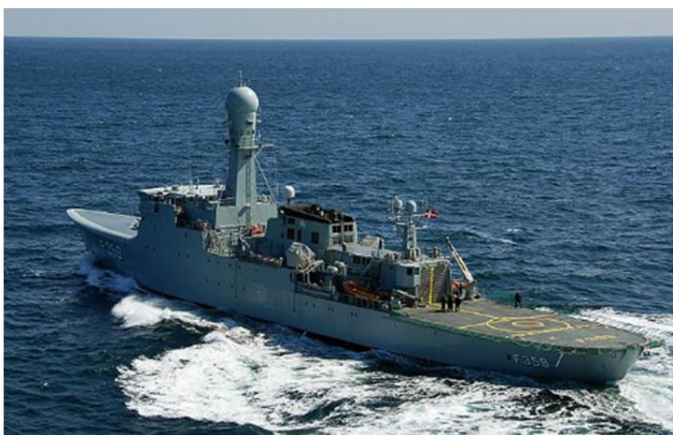
Figure 5-19. HMDS Vædderen , a 3500-ton displacement ice-strengthened patrol vessel of the Danish Coast Guard (USCG photo). 1
