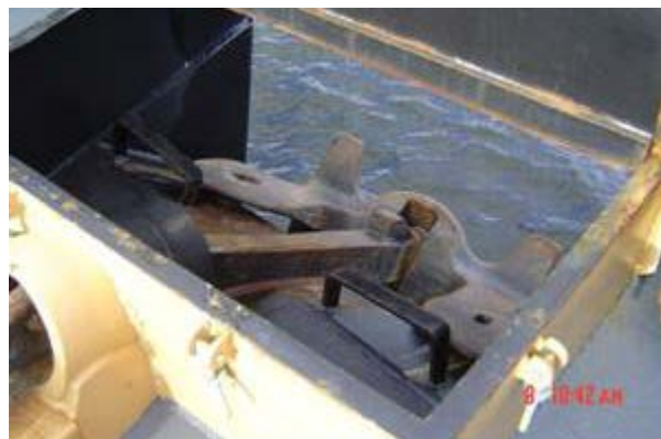
Figure 4-58. Anchor hardware that ices on the foredeck (CRREL 2012).
