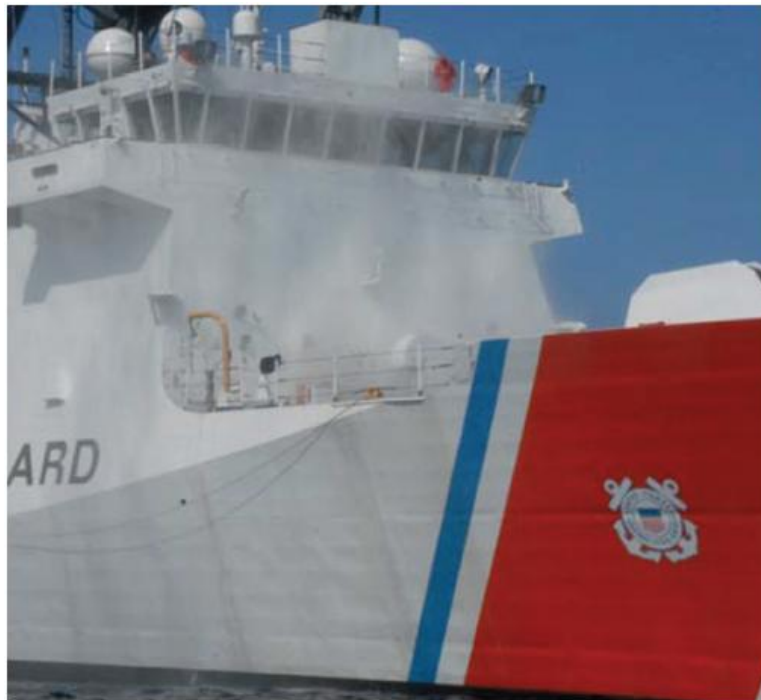
Figure 5-2. Countermeasure Washdown System in operation on CGC BERTHOLD (Coast Guard photo).
