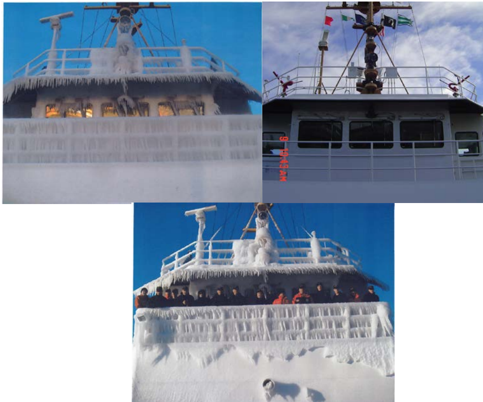
Figure 4-59. Iced bridge and flying bridge on CGC BISCAYNE BAY in Lake Superior (upper left). Ice free bridge and flying bridge on CGC THUNDER BAY for comparison (upper right). Bottom image shows height to which de-icing can occur from the forecastle deck. (CGC BISCAYNE BAY photos courtesy LCDR Godwin, USCG; CGC THUNDER BAY photos by CRREL 2012).
