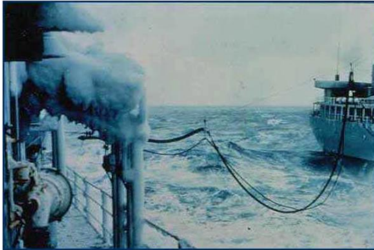
Figure 7-5. UNREP during superstructure icing conditions (National Ice Center 2001).
