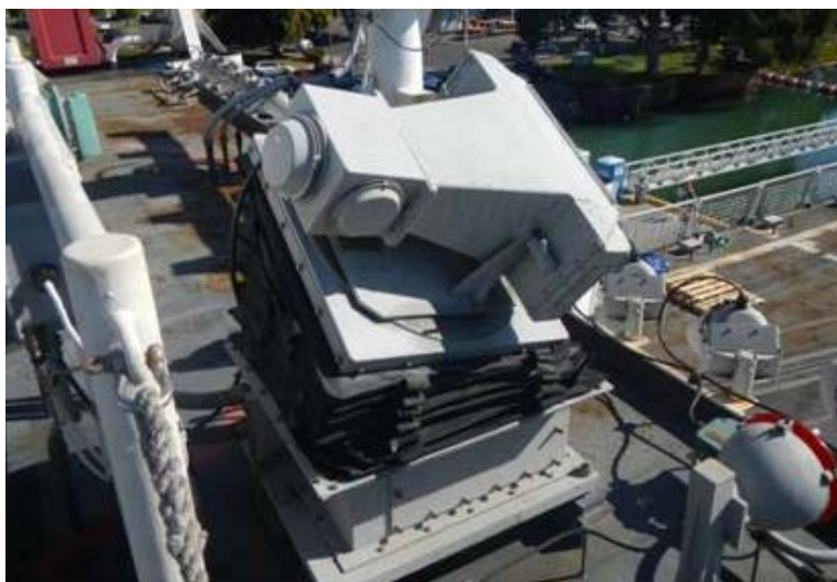
Figure 4-45. Visual approach slope indicator for helicopter landings on flight deck. Bellows icing could hinder movement or puncture bellows (Ryerson 2012).
