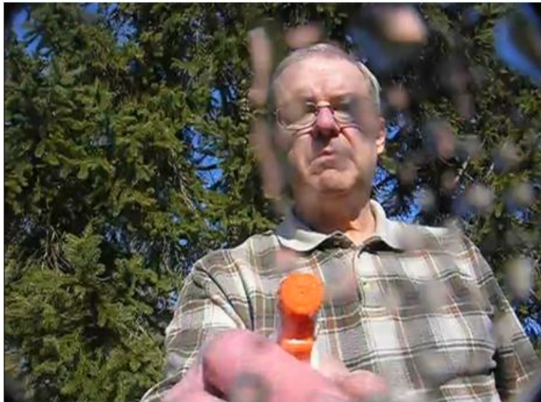
Figure 5-52. Window being sprayed with water. Left side of image is coated with Oak Ridge National Labs transparent coating and right side is uncoated.
