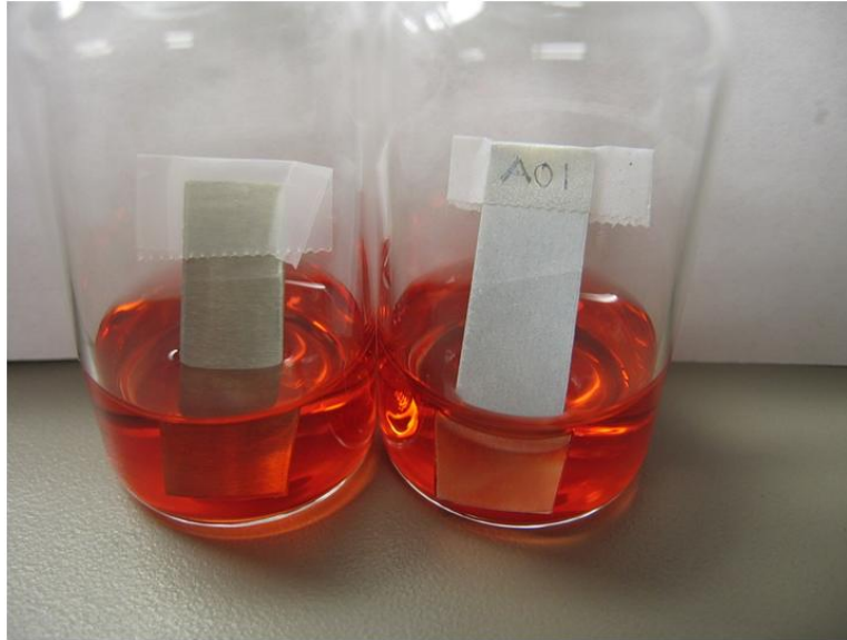
Figure B-7. Start of corrosion test with ISurTec-coated aluminum on right, bare aluminum on left.
