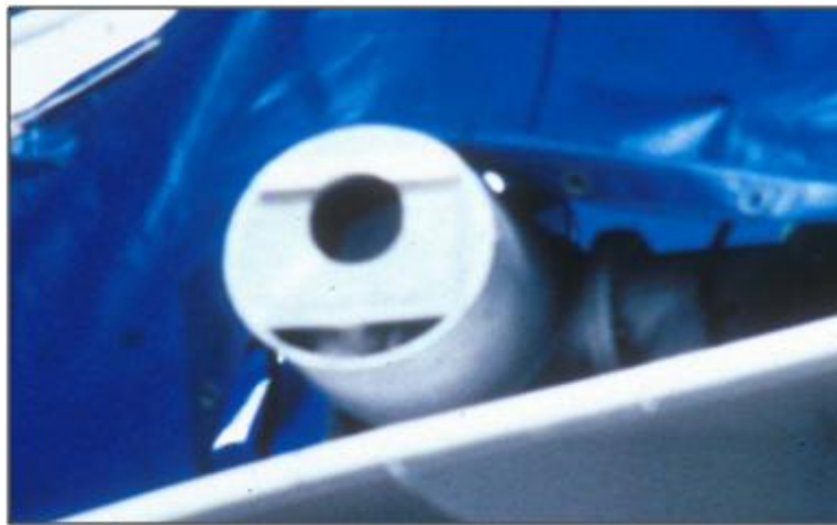
Figure 5-50. Camera housing window with glass perimeter electrically heated on CGC MIDGETT (Ryerson 1990).
