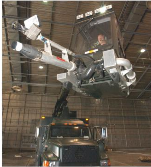
Figure B-32. Air Force Global AirPlus! system. Larger nozzle blows air or air and de-icing fluid mist (bottom). Smaller nozzle sprays de-icing fluid at low velocity (top).
