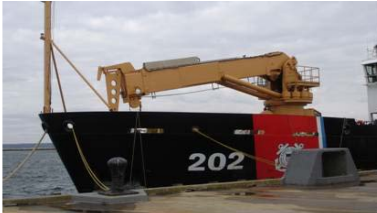
Figure 4-75. Sheets of ice can fall from the crane after icing. The crane is parked over the buoy deck when in transit, 180° from view above, which makes falling ice a hazard when that deck is used before de-icing the crane (Ryerson 2012).
