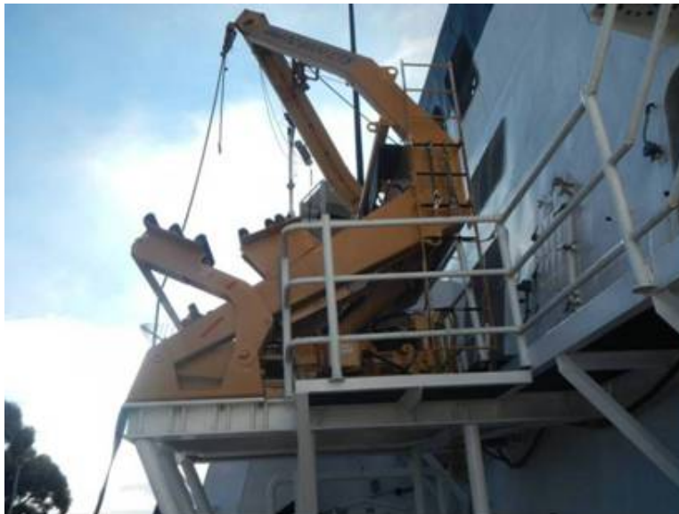
Figure 4-34. Single davit for launching boat, located one level above boat deck. It is understood that little spray reaches this height, but it is a complex machine that is difficult to keep operating fully in less severe conditions than icing (Ryerson 2012).
