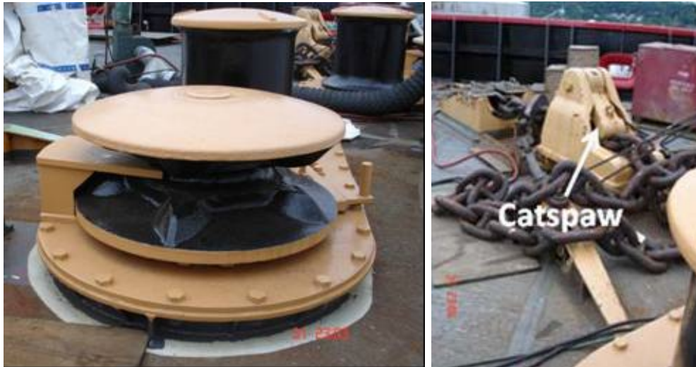
Figure 4-10. Anchor hardware including wildcat on left and catspaw on right (CRREL 2012).
