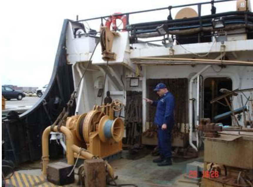
Figure 4-74. Officer indicating windlass and aft-facing bulkhead area at forward end of buoy deck that ices heavily from sea spray (Ryerson 2012).
