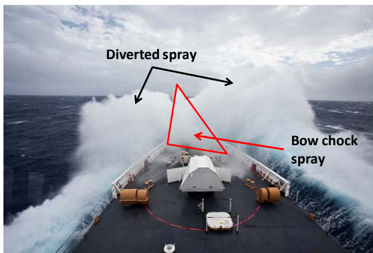
Figure 4-22. Spray diverted away from bow by flare in heavy seas. Note, however, water jetting through the bow chock and wetting the deck (courtesy LCDR Reid, CGC WAESCHE 2012).
