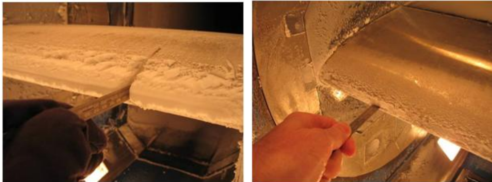
Figure B-36. (Left) An airfoil specimen exposed to realistic impinging ice conditions in Goodrich's wind/ice tunnel. Ice forms on the leading edge with no ice protection. (Right) Same airfoil exposed to the same icing conditions but with the ultrasonic ice protection system turned on. Note only a thin film of ice is formed on the leading edge. The actuators are embedded inside of the leading edge (not shown).
