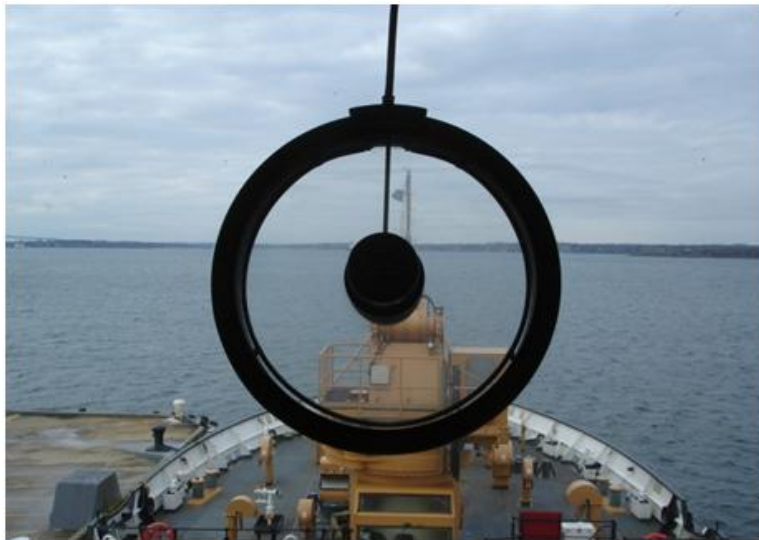
Figure 5-53. Spinning window on bridge of the 225-ft seagoing buoy tender CGC WILLOW (Ryerson 2012).
