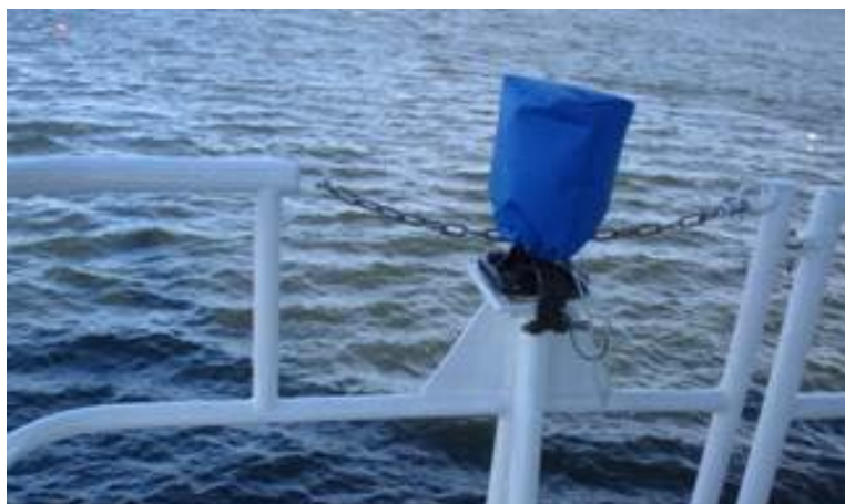
Figure 4-66. Gun mount covered with tarp to reduce icing and other weather effects (CRREL 2012).
