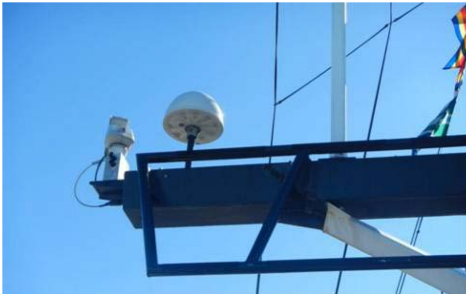
Figure 4-51. Starboard mast lower cross arm with camera and antennas (Ryerson 2012).
