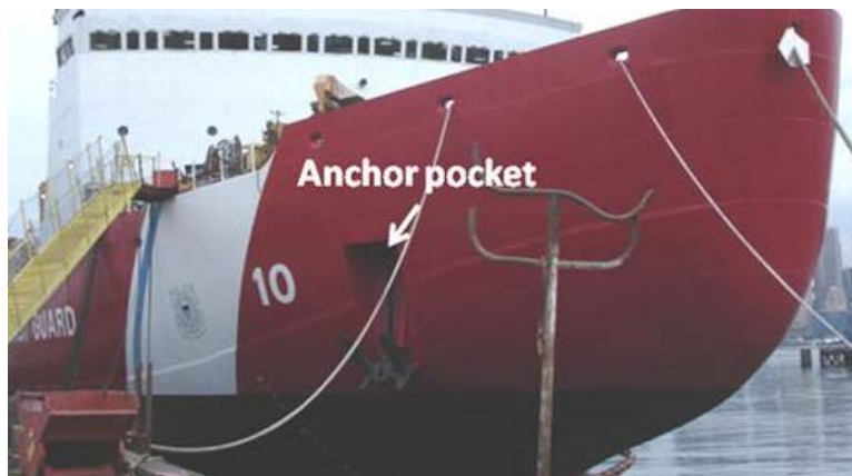
Figure 4-11. Anchor can freeze when drawn into anchor pocket and not release when required (CRREL 2012).
