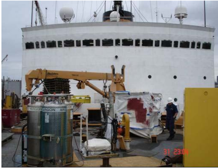
Figure 4-12. Manual de-icing techniques cannot reach high on forward bulkhead causing a falling ice hazard. Ice can also fall from the crane (CRREL 2012).
