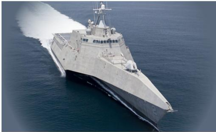
Figure 5-16. US Navy littoral combat ship USS Independence with trimaran hull with significant rake and tumblehome (US Navy).
