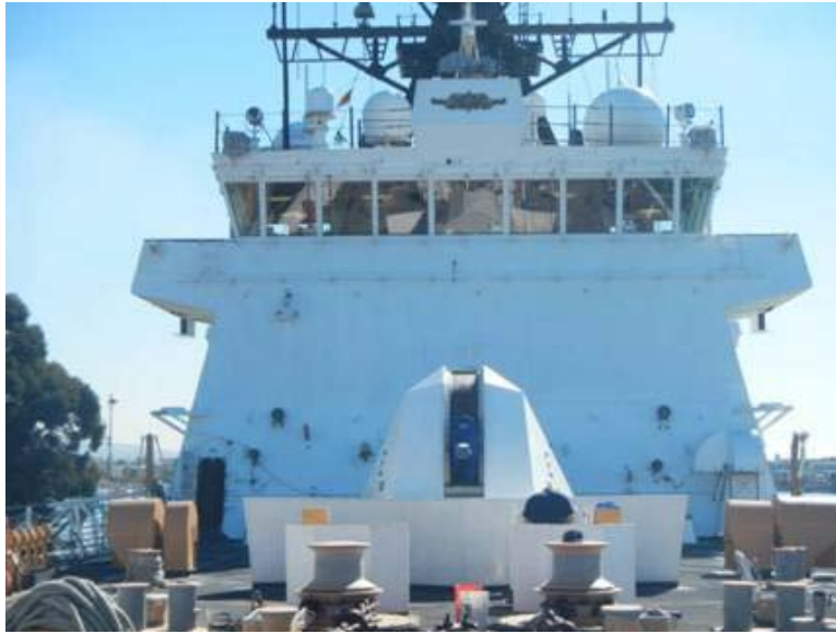
Figure 4-32. The 57-mm gun turret is a composite structure and could be damaged by manual de-icing. The spray shield below and forward of the gun may accumulate ice at its base and hinder forecastle deck drainage (Ryerson 2012).
