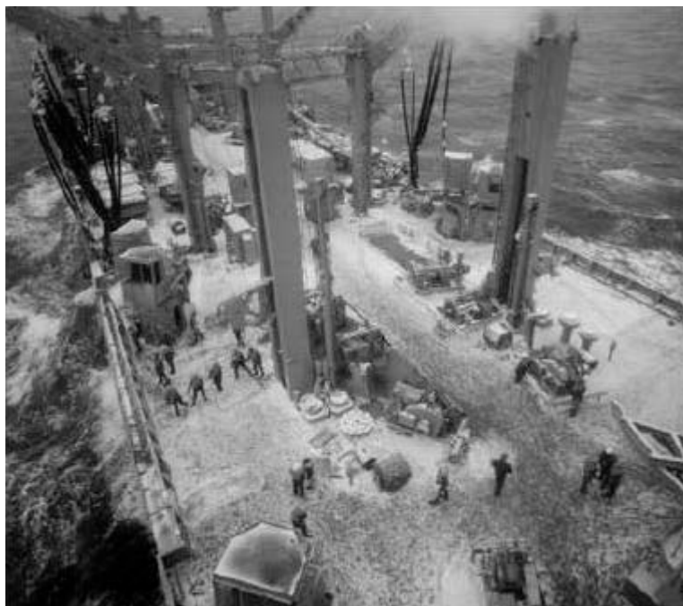
Figure 3-25. Navy UNREP tests in the Bering Sea, 1977, on the USS Roanoke , a replenishment oiler. Decks are snow and ice-covered (from Miller 2009).
