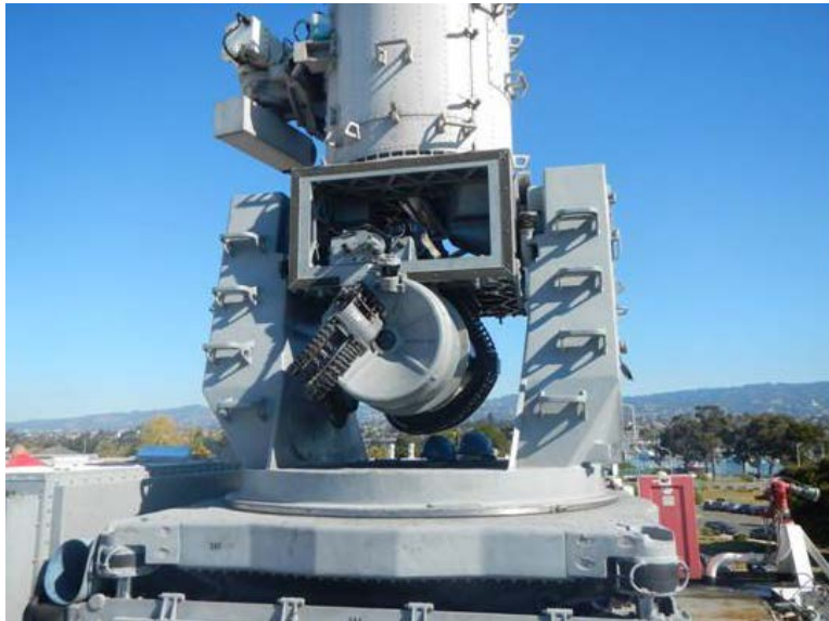
Figure 4-44. CWIS system is located on the port side on top of hangar. Exposed ammunition belts that feed rounds from barrel below gun could jam in icing conditions (Ryerson 2012).
