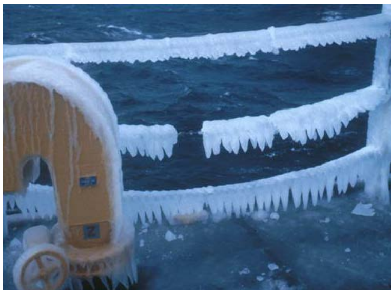
Figure 3-20. Lifeline vertical ice sample on the CGC MIDGETT (Ryerson 1990).
