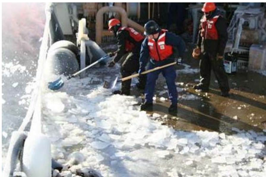
Figure 4.83. Removing about 2–5 cm of fresh-water ice from the CGC ALDER'S buoy deck using shovels and wooden mallets. Note the personal protection equipment necessary for safety ( http://www.uscg.mil/d9/cgcAlder/Photo_gallery.asp ).
