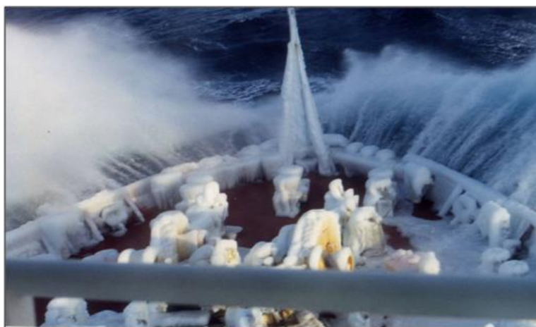
Figure 5-33. Though the deck hardware and bulwarks are freezing, and even the scuppers are frozen shut, sufficient water is flowing over the deck to keep it largely free of ice. Heat from below decks could also be a contributing factor (from CRREL).
