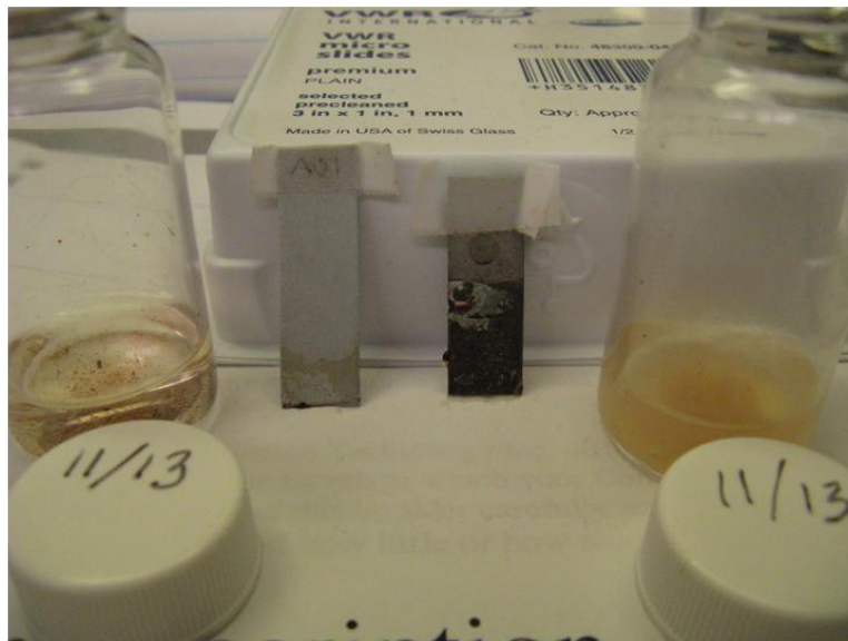
Figure B-8. After 1 year of immersion, the bare aluminum coupon (right) is well-corroded, and the ISurTec-coated coupon (left) has minimal corrosion.
