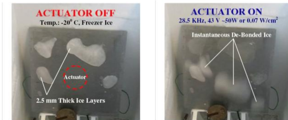
Figure B-35. Ice bonded to plate top, with actuator location indicated on back of plate. Instant of ice debonding and falling upon activating actuator (Palacios et al. 2008).
