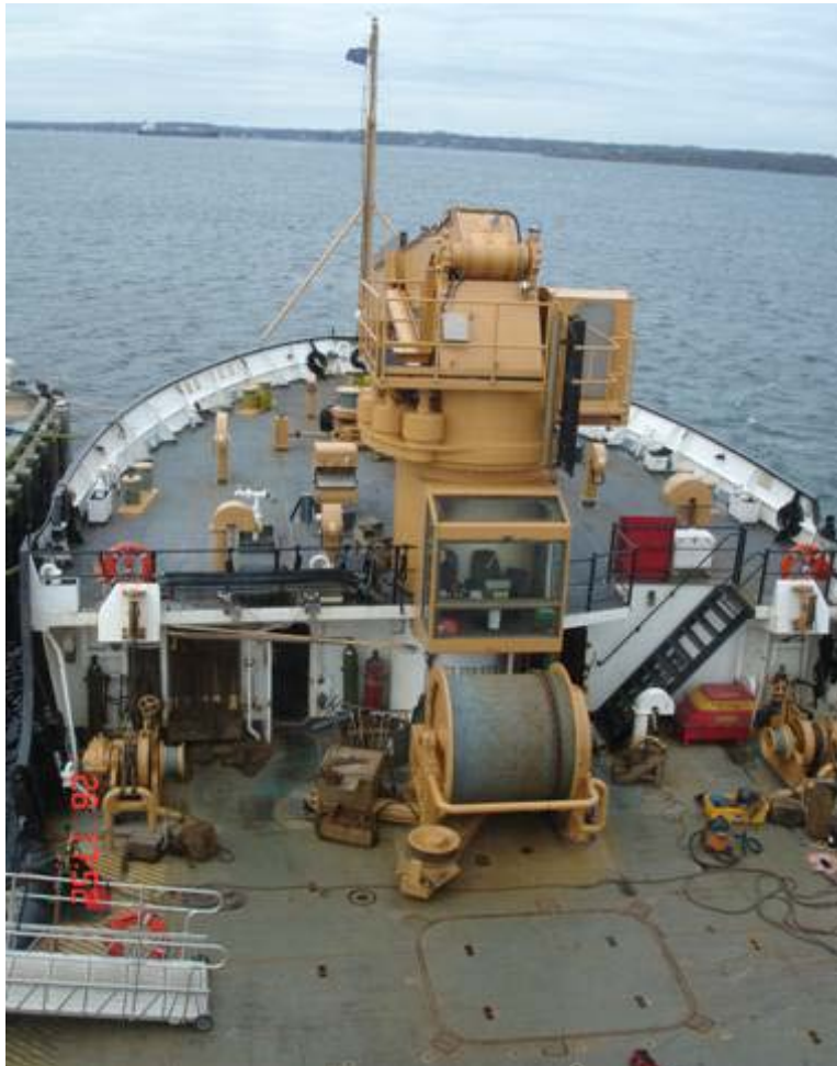
Figure 4-70. Forecastle (forward) covered with non-skid, and the zinc-covered buoy deck (aft) of the CGC WILLLOW. The crane is rotated 180° when the vessel is in-transit (Ryerson 2012).
