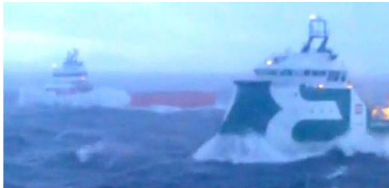
Figure 5-18. X-bow in foreground generally creates less spray than conventional bow in background, which was moving more slowly than the foreground ship. 1
