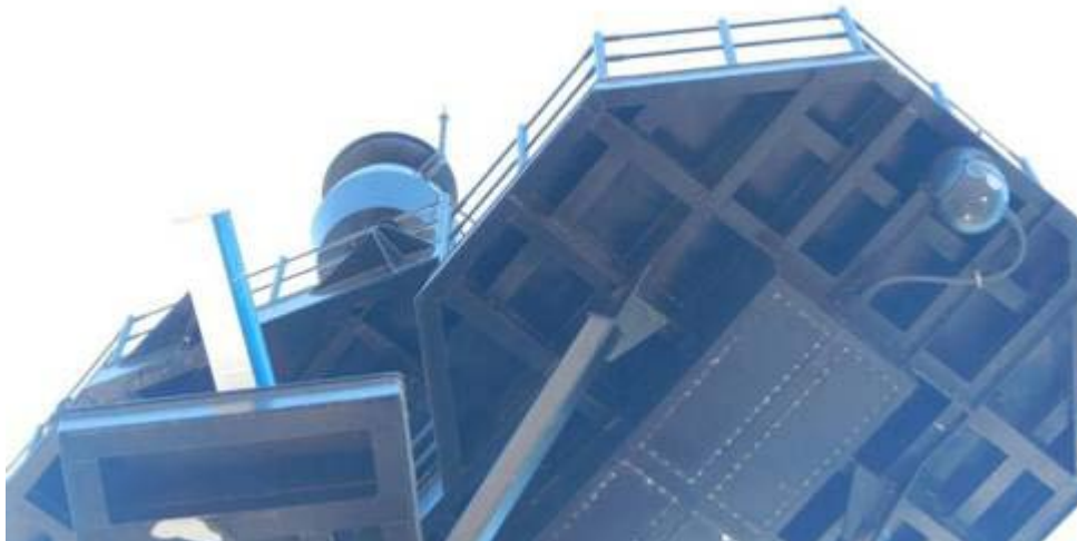
Figure 4-53. Radar antenna (left), sensor under platform (right), and radar system on topmast (Ryerson 2012).
