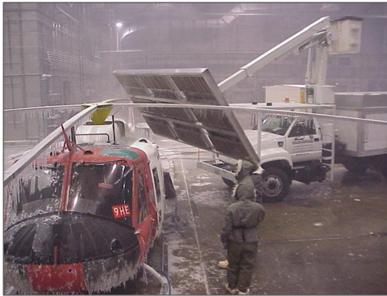
Figure 5-40. Ice Cat de-icing helicopter tail boom in Eglin Air Force Base McKinley Climatic Chamber (Ryerson).
