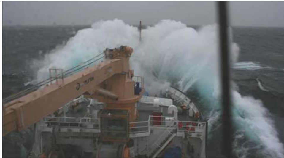
Figure 4-69. Bow plunging and spray generation on the CGC ALDER. Note the white spray shield on the deck ahead of the crane. The CGC WILLOW has no forecastle spray shield, but icing experience suggests that it is desirable ( http://www.uscg.mil/d9/cgcAlder/photo_gallery.asp ).
