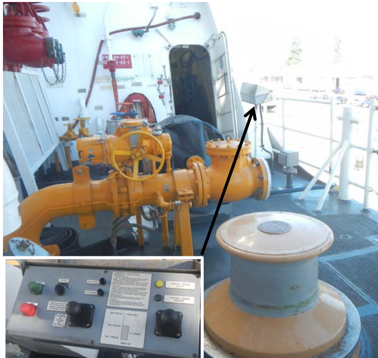
Figure 4-33. The boat deck has considerable hardware, operations involve several personnel, the area receives spray, and icing is expected. Inset shows single davit control station, and arrow shows control station location—on a deck that may be iced (Ryerson 2012).
