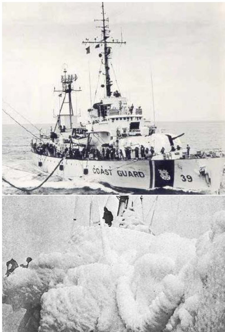
Figure 3-28. Top—CGC OWASCO (US Coast Guard 2013). Bottom—starboard side of CGC OWASCO after accumulating up to 25 cm of ice at Ocean Station "Bravo" (DeAngelis 1974).
