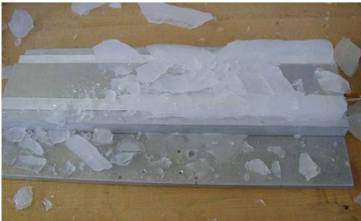
Figure B-25. Single actuator under 3.2-mm metal plate with 25-mm ice sheet (top). Actuator breaking ice sheet (bottom). (Images courtesy Innovative Dynamics Inc.)
