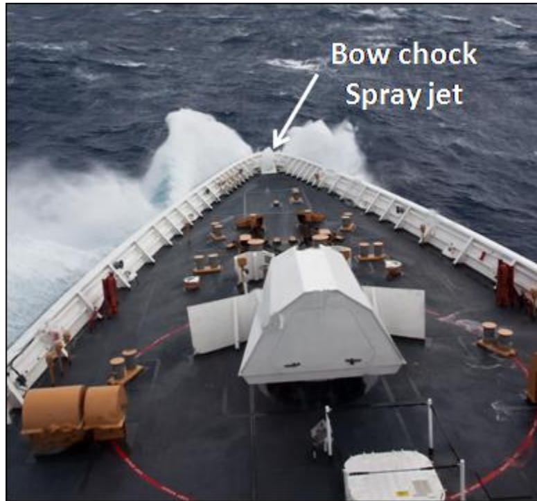
Figure 3-2. Initial plunging of NSC WAESCHE bow in 35- to 40-kt (18- to 20-m/s) winds and 3.5- to 6-m seas with a ship speed of 18 kt (9 m/s) during Tropical Depression Haikui. The beginning of a spray jet is entering the forecastle through the bow chock (courtesy LCDR Reid, CGC WAESCHE 2012).
