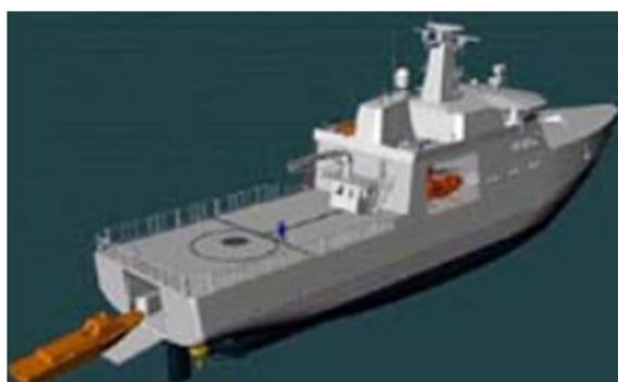
Figure 5-21. Danish Knud Rasmussen -Class inspection ship with stern covered small boat launch and recovery system (image courtesy Defence Command Denmark).
