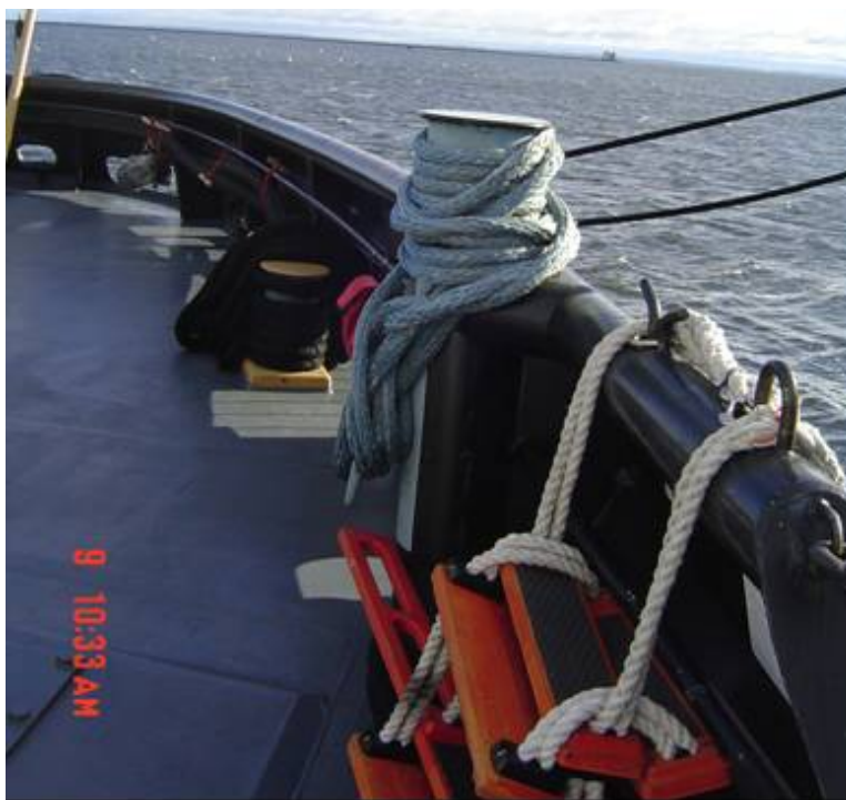
Figure 4-65. Synthetic line (wound around cleat) freezes hard; double braided line on ladder stays flexible in cold weather (CRREL 2012).
