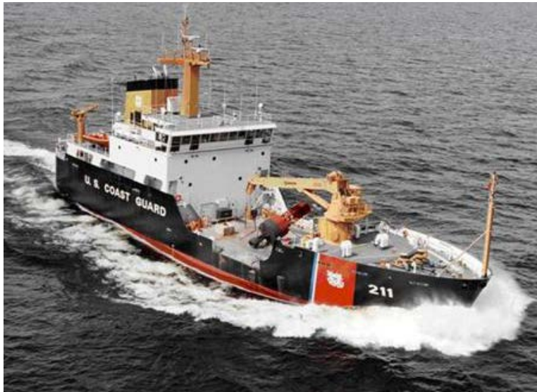
Figure 4-67. CGC OAK showing spray generated in calm seas and forecandle crane in parked position over buoy deck when underway (US Coast Guard, n.d.).
