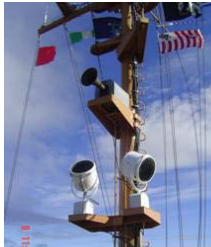
Figure 4-60. Spray and icing reached the ships horn about 15 ft above the flying bridge on the CGC BISCAYNE BAY (see Fig. 4-59). This photo is of the CGC THUNDER BAY (CRREL 2012).
