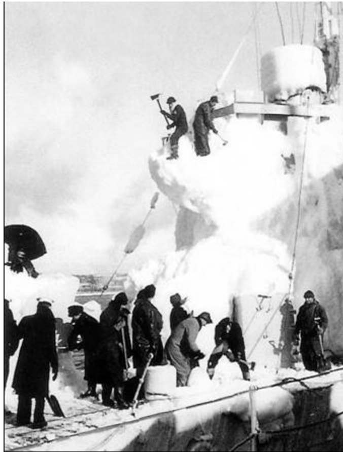
Figure 3-29. De-icing bridge and forecandle of HMS Leamington in 1943 using tools not dissimilar to those used today. Photo courtesy of Phil Marley ( www.hazegray.org/navhist/canada/bota/m/leamington/ )
