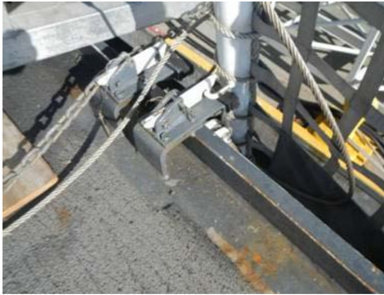
Figure 4-37. Latches for flight ops rescue team nets involve pulling pins that could freeze, making removal difficult (US Coast Guard 2012).
