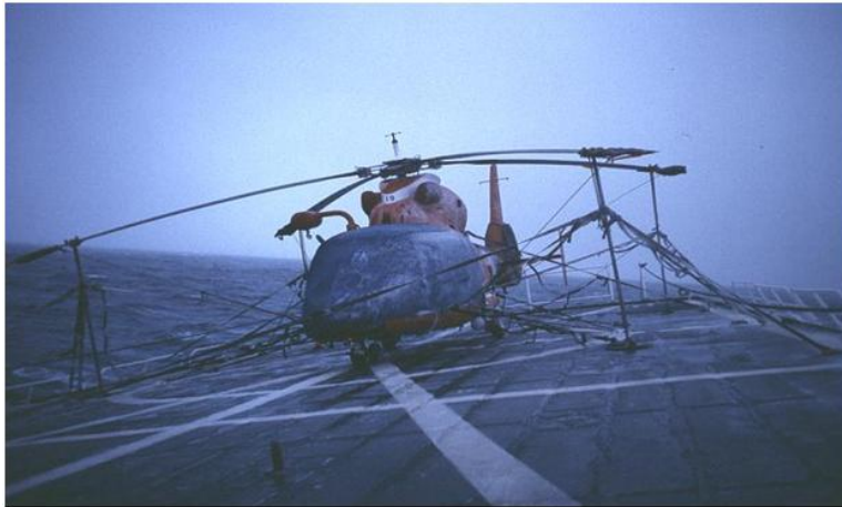
Figure 5-14. Coast Guard Dolphin helicopter with fitted tarps covering windscreen, engine intakes, and ducted tail fan on CGC MIDGETT, 1990 (Ryerson).
