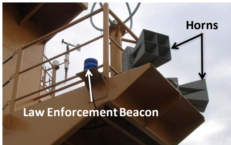
Figure 4.76. Incandescent Law Enforcement beacons stay deiced when in operation, but may not if converted to LEDs. Horns on mast fail in snow, freezing rain and sleet (Ryerson 2012).
