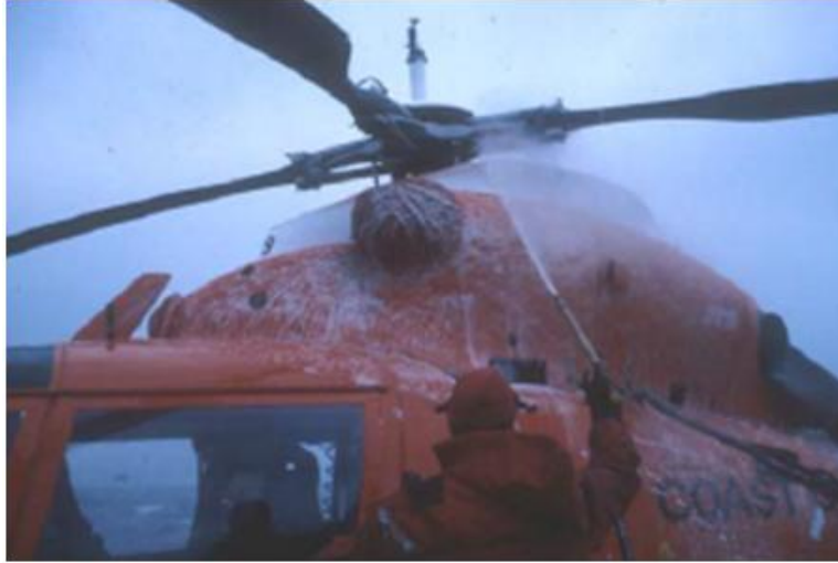
Figure 5-35. Coast Guard helicopter being de-iced with a heated pressure washing system using a de-icing fluid. Note the engine inlet covers (Ryerson).
