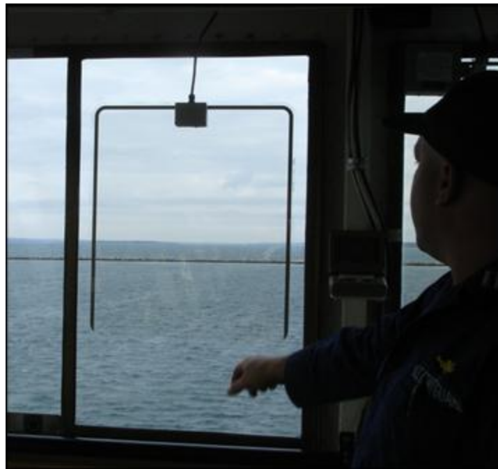
Figure 4-84. Seaclear after-market adhesive electric window heater to replace failed window heaters (Ryerson 2012).
