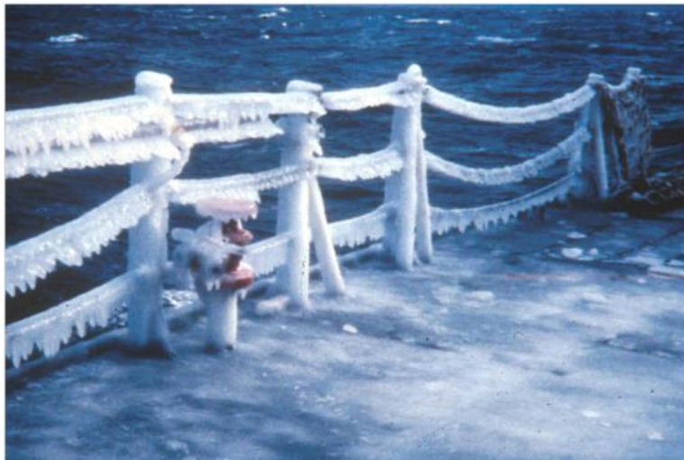
Figure 5-54. Sea spray ice on CGC MIDGETT cable lifelines (Ryerson 1990).
