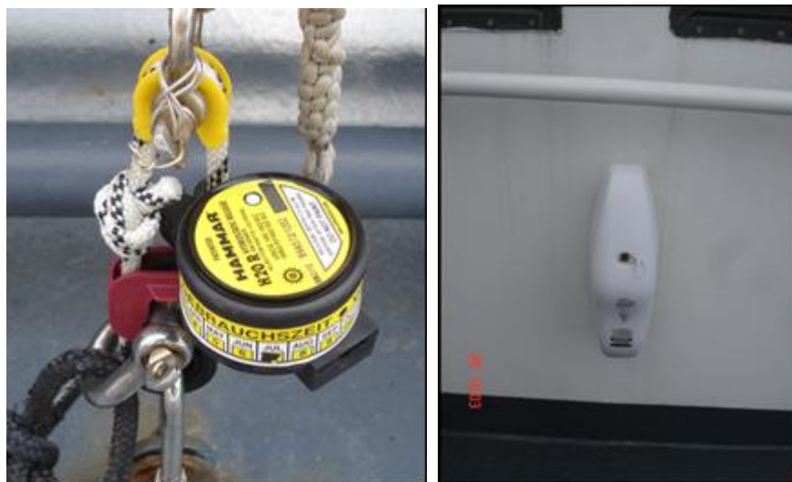
Figure 4-81. Hydrostatic life raft releases can ice and fail if vessel sinks (left), and EPIRBs can freeze in-place and not release if vessel sinks (right) (Ryerson 2012).
