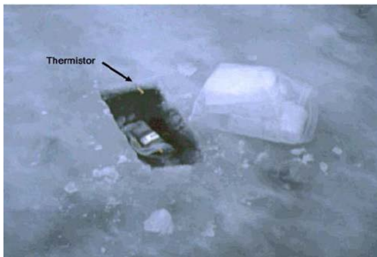
Figure 3-19. Ice samples in a freezer bag, and a thermistor for measurement of in situ ice temperature (Ryerson 1990).
