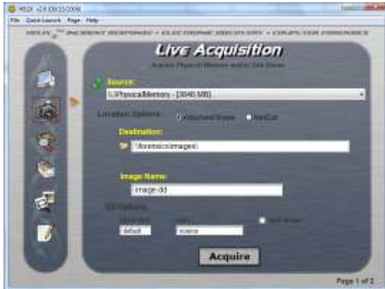
Figure 3 Live Acquisition Using dd
