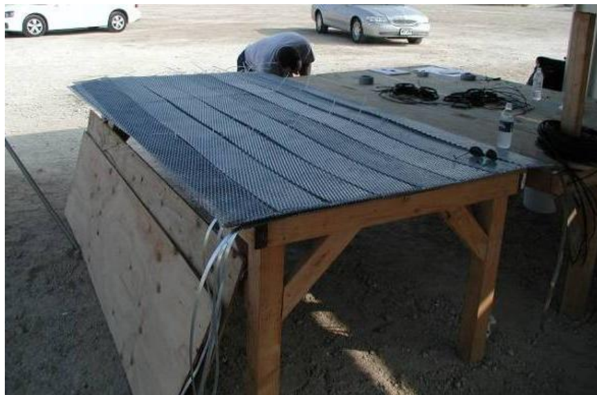
Figure 6. Assembled apron of eight mesh anode strips.
