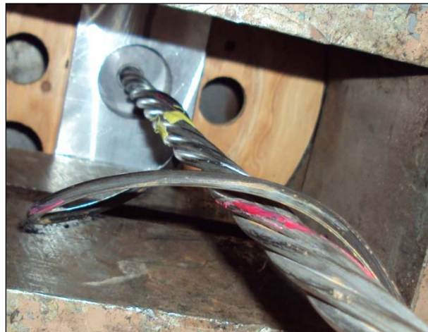
Figure 8-11. Cable unwinding due to energy release after failure.
